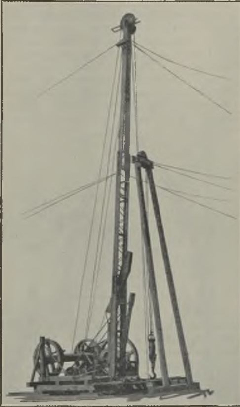
FIG. 8.—PORTABLE DRILLING RIG, CAPABLE OF DRILLING TO 2,500 FT. SHEAR-LEGS FOR HANDLING CASING ARE SHOWN.
