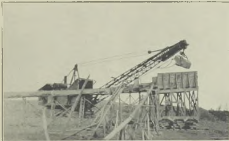
FIG. 7.—DRAGLINE PLACER MINING IN ALASKA.
