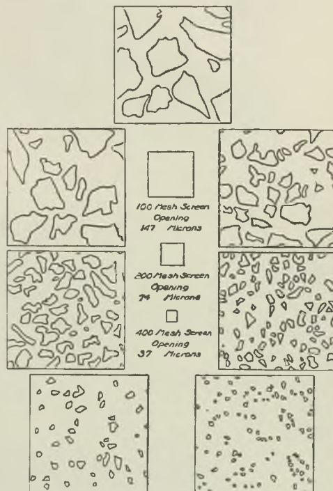
FIG. 2.—ELUTRIATED PRODUCTS OF ZINC CONCENTRATE.
