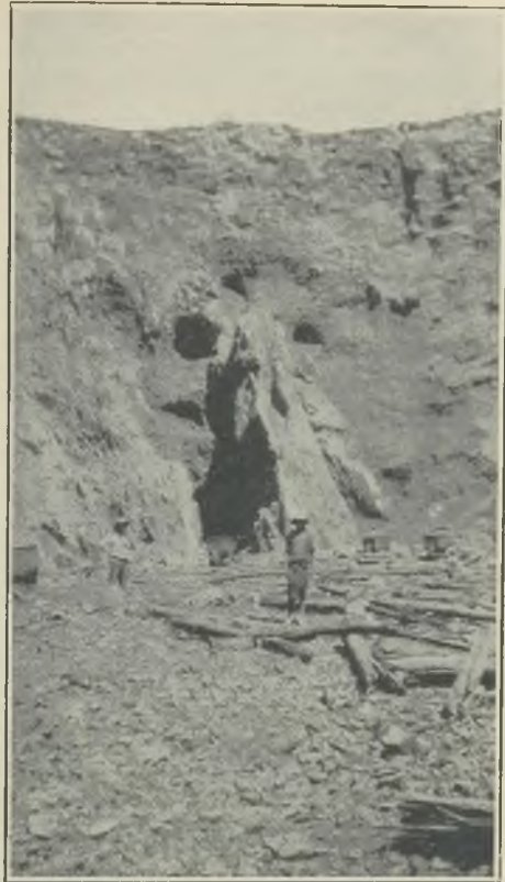
OPEN-CAST AT ABENAR MINE: SHOWING PLATY LIMESTONE (FOOTWALL) ON THE LEFT AND BRECCIA ON THE RIGHT.
