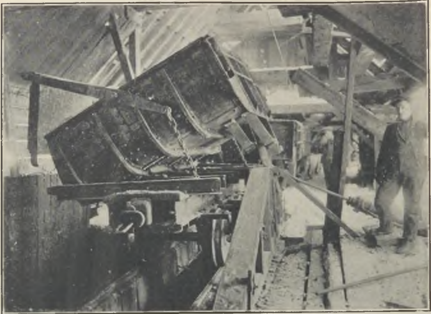
FIG. 4.—10-TON CAPACITY GRANBY CAR WITH FREE-SWINGING DOOR TO PASS LARGE PIECES OF ORE.
