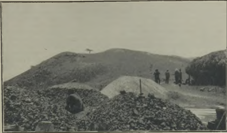
FIG. 13.—THE SURFACE AT MWIRASANDU TIN MINE; THE HEAPS OF MATERIAL ARE COMPOSED OF ELUVIAL TINSTONE, HAND-GATHERED FROM THE SOIL.
