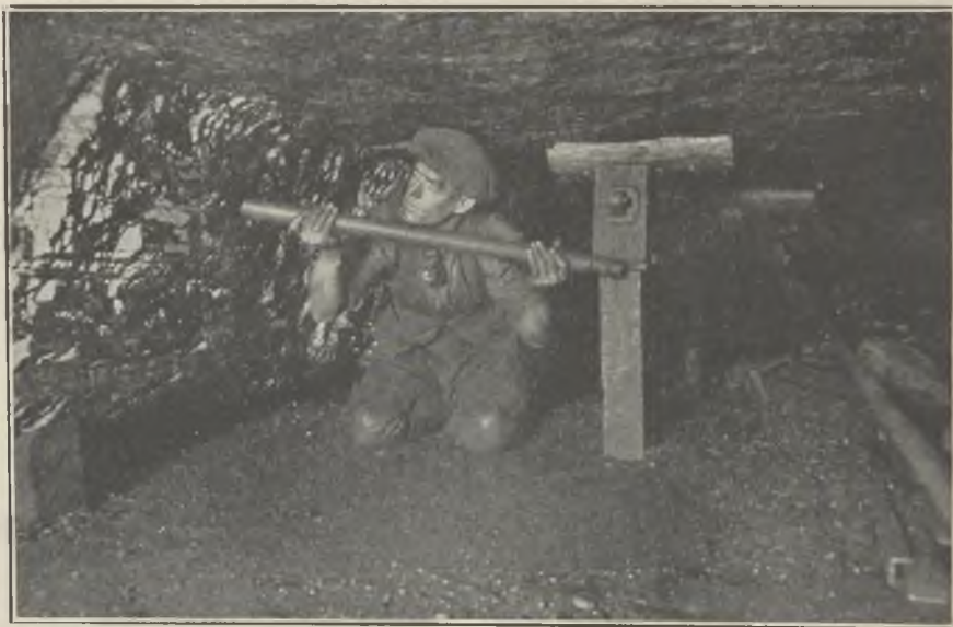
FIG. 4.—INSERTING THE CARDOX SHELL IN HOLE.
