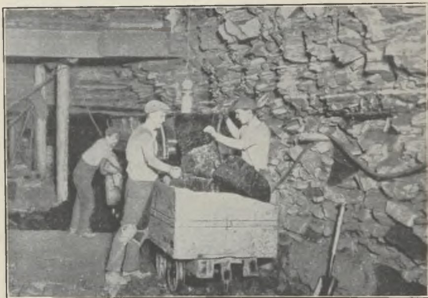
FIG. 7.—LOADING CARDOX-SHOT COAL INTO TUBS AT GATE-END LOADER.
