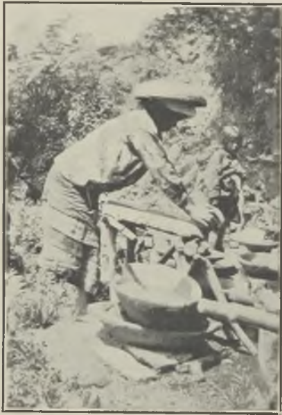
FINE GRINDING ON A RUB-ROCK.
