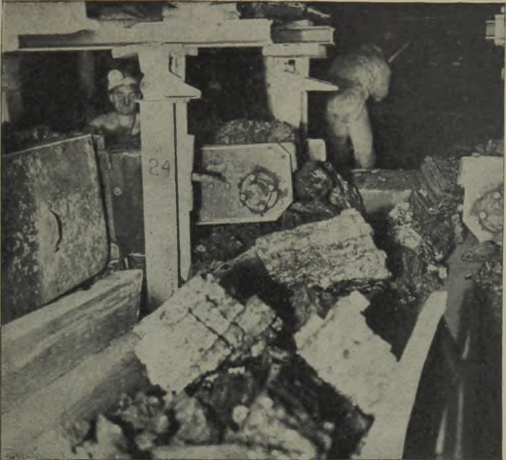
DUNLOP Face belts delivering to Gate belt at the Manchester Colliery Company's Workings
