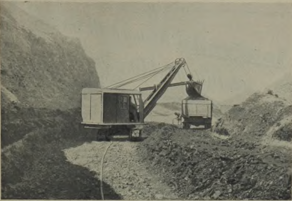
The 24-RB Electric Shovel shown here has a \frac{7}{8} yard dipper and is excavating and loading opencast coal.
