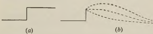
Fig. 2.—Unit step impressed on the first grid gives these fundamentally possible responses. They all tend to zero.
