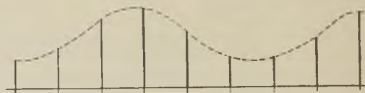
Fig. 13.—In “pulse modulation” the curve is chopped at equal intervals of time by sharp pulses.
