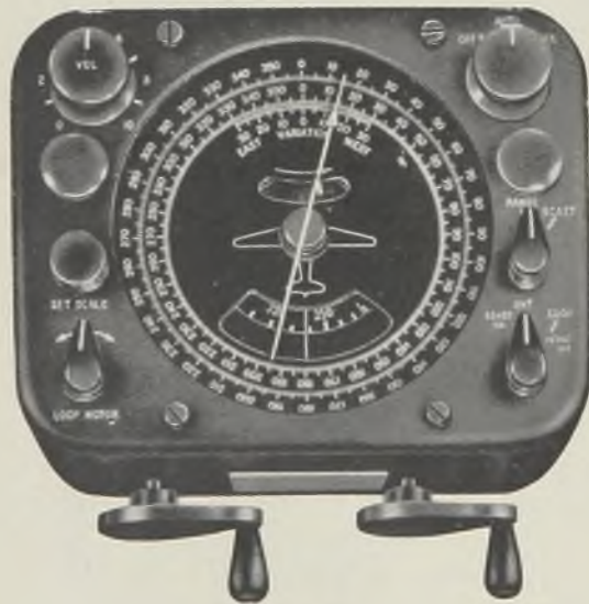
Automatic radio compass presentation and remote control unit. (Sperry gyroscope photograph.)
