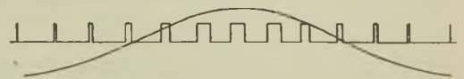
Fig. 15.—Signal and corresponding "variable width modulation." The variable width modulation is usually derived from the time modulation at the receiver.
