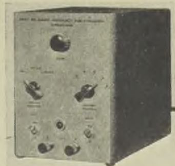
Quartz Crystal Calibrator, Mains Driven, Modulated when Desired, 10, 100 and 1000 kc.s. Markers.
