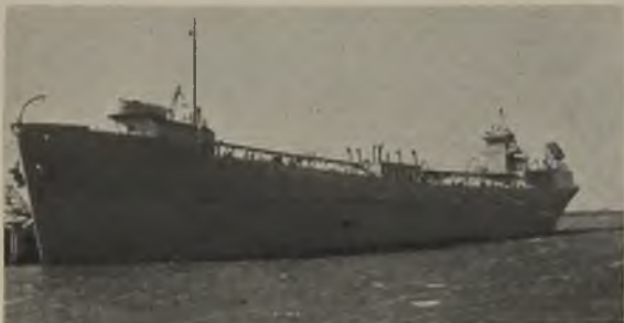
Fig. 1—One of four concrete oil barges built at Houston. Seven similar tankers were built at Savannah.
