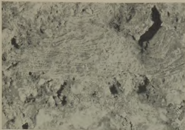
Fig. C—Ice segregation resulting from slow freezing starting when the concrete was 4 hours old—magnified 4\frac{1}{2} x
