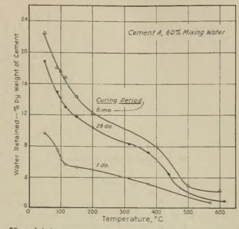
Fig. 9 – Effect of drying temperature on water retained, temperature range 50 to 600C Wilson and Martin, J. Am. Concrete list. v. 31, p. 272 (1935)
