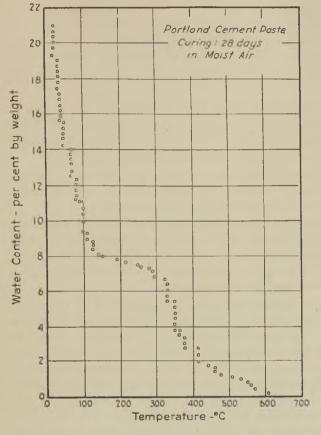
Fig. 13 – Isobar for portland cement paste obtained by Krauss and Jorns.
