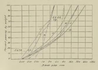
Fig. 4—Sieve analyses of aggregates used in test specimens.
