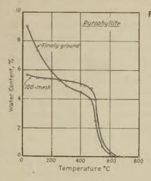
Fig. 5 – Isobar for pyrophyllite Data from Kelley, Jenny and Brown Soil Sci. v. 41, p. 260 (1936)
