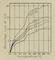
Fig. 10—Loss-on-heating curves for hardened neat cement, w/c=0.22 Lea & Jones, J. Soc. Chem. Ind., v. 54, p. 63, 1935
