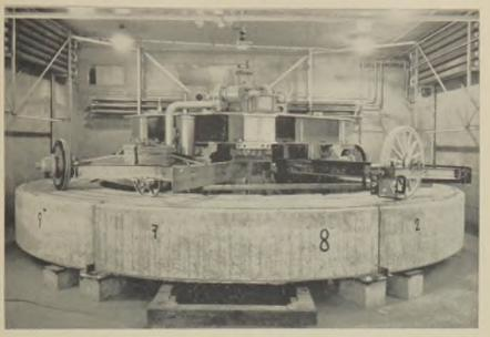
Fig. 2--Road testing machine during wear tests. At left is shown one of the two driving wheels, left center a steel truck wheel and at right a leather-covered wheel.
