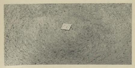
Fig. 6—Test specimen 10. Vibrated concrete floor. Mix by weight 1:3.2:4.3, w/c ratio 0,51, consistency 26 vebe-degrees. This photograph was taken immediately after wood-floating.
