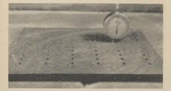
Fig. 7 — Measuring the depth of wear by inserting a dial indicator into a hole in a steel plate.
