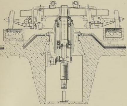
Fig. 3-Cross-sectional view of the road testing machine in normal operation.
