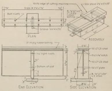
Fig. 1—Apparatus for testing silo staves
