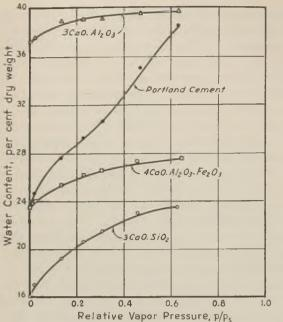
Fig. 19 – Water content vs. vapor pressure relationship Berchem, Diss. Eidg. Techn. Hochschula, Zurich (1936)
