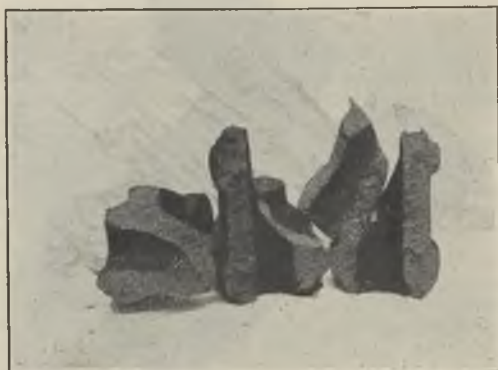
FIG. 12.—THE CASTING SHOWN IN FIG. 11, BROKEN UP TO EXHIBIT THE SOLIDITY.
