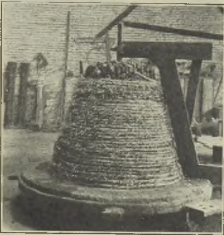
FIG. 4.—THE WITHDRAWN CORE REMADE WITH STRAW ROPE AND—ON THE TOP—COKE. IT IS NOW READY FOR STRICKLING.
