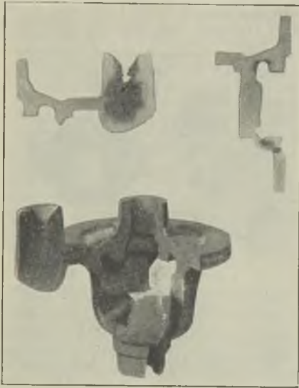
FIG. 13.—A CASTING DIFFICULT TO MANUFACTURE OWING TO THE VARYING THICKNESSES OF METAL.
