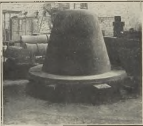
FIG. 1.—FINISHED CORE FOR SLAG POT.
