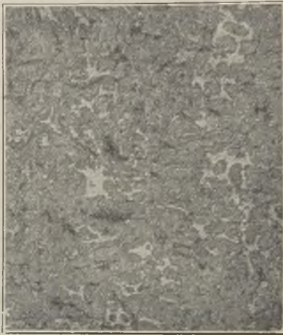
FIG. 3.—SEMI-STEEL MAGNIFIED 100 DIAS. BUT REDUCED ON REPRODUCTION. IT CONTAINS 1.03 PER CENT. P.
