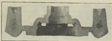
FIG. 16.—HALF OF CASTING FED BY TWO RISERS AND MADE SOUND BY THE INTRODUCTION OF A STRAP.
