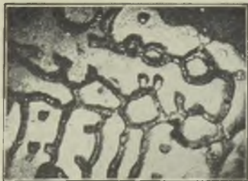
FIG. 2.—MICRO-SECTION OF A ROLLED COPPER BAR SHOWING THE EFFECT OF OXYGEN.
