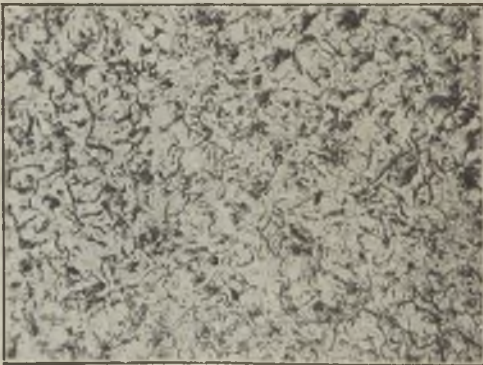
FIG. 2.—MICRO-STRUCTURES OF SEMI-STEEL. THE UPPER IS ETCHED AND MAGNIFIED AT 250 DIAS. AND THE LOWER UN-ETCHED AND MAGNIFIED 110 DIAS.
