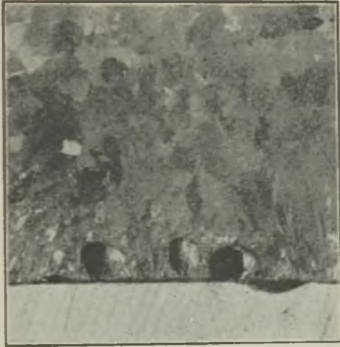
FIG. 6.—INFLUENCE OF CHILL TEMPERATURE ON GRAIN GROWTH ALMOST DESTROYED.
