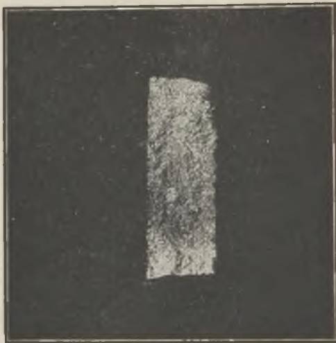
FIG. 9.—FRACTURE OF CHILLED IRON, WHITE IRON GRADUALLY MERGING INTO GREY IRON.
