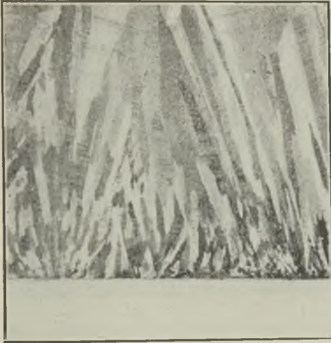
FIG. 2.—GRAIN GROWTH AS INFLUENCED BY LIGHT CHILL.
