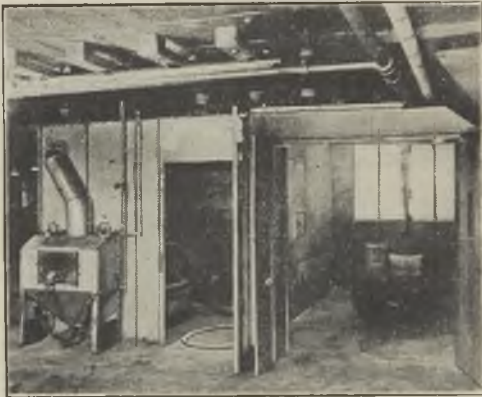
FIG. 15.—COMBINATION SAND-BLAST ROOM AND CABINET.
