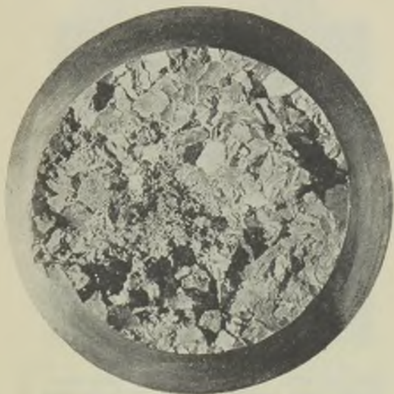
FIG. 7.—FRACTURE OF A HIGH TENACITY "BETA" BRASS VALVE ON A HYDRAULIC PRESS.
