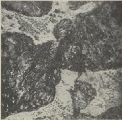
FIG. 1.—MATRIX CONSISTING OF WELL-DEFINED LAMINATED PEARLITE.
