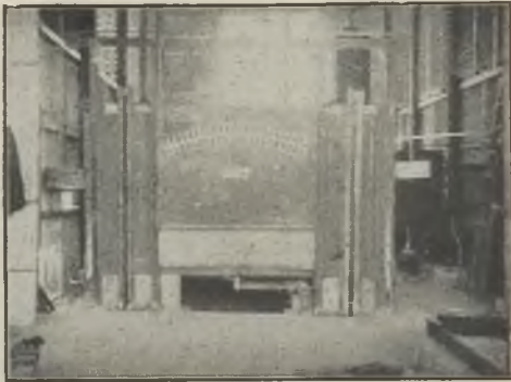
FIG. 10.—GAS-FIRED REVERBERATORY MELTING FURNACE.
