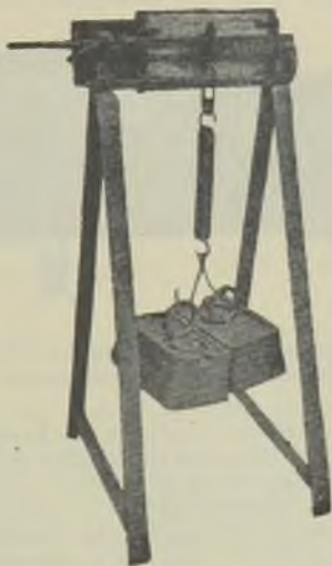
FIG. 8.—LEVER-ACTUATED MACHINE FOR SHEAR-TESTING CAST-IRON.
