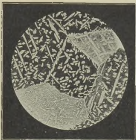
FIG. 9.—EFFECT OF SUBSTITUTING 1 PER CENT. AL. FOR SAME AMOUNT OF ZN. IN A 59 PER CENT. COPPER-BRASS.
