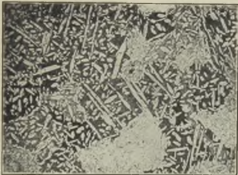
FIG. 11, SHOWING MICROSTRUCTURE OF ALLOY AM5 "AS CAST."
