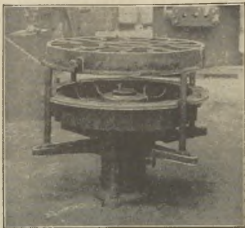
FIG. 18.—A WHEEL PATTERN MOUNTED ON A MOULDING MACHINE.
