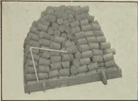
FIG. 2.—CAST-IRON BRIQUETTES MADE FROM BORINGS AND BONDED WITH CLAY WASH.
