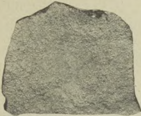
FIG. 3.—FRACTURE OF AN IRON WHICH CONTAINED 4.25 PER CENT. SILICON.
