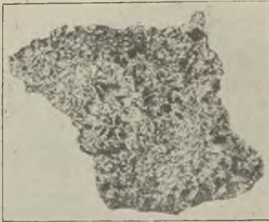
FIG. 4.—SAMPLE OF UNDRILLABLE PIG-IRON OF NORMAL ANALYSIS.
