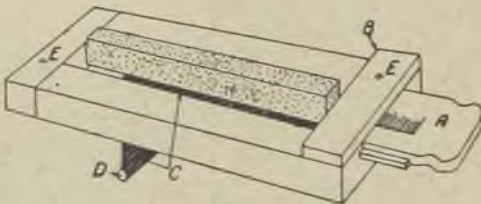
FIG. 3.—APPARATUS FOR TESTING GREEN BOND STRENGTH.
