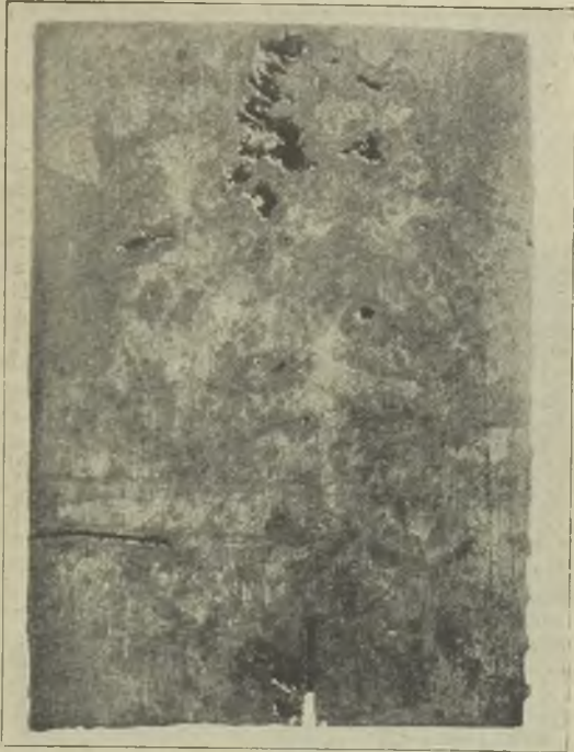
FIG. 13C.—SEGREGATION IN A PROPELLER SHAFT LINER CASTING, MAG. 5 DIAS.
