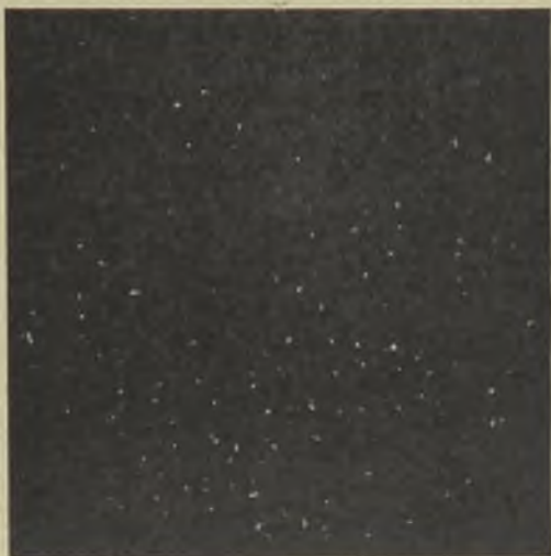
FIG. 7.—DELTA EUTECTOID IN GOOD GUNMETAL, SHOWN IN FIG. 5. \times 50 .
