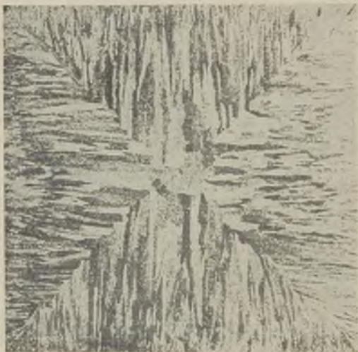
FIG. 7.—SHOWING COLUMNAR CRYSTALS ACROSS A SECTION OF THE CASTING.
