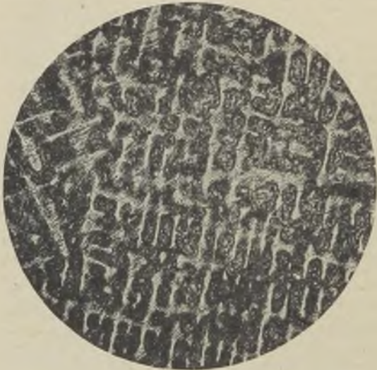
FIG. 1.—STRUCTURE OF GUN-METAL AT 100 DIAS. TO BE ASSOCIATED WITH A GOOD METAL.
