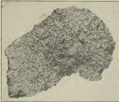
FIG. 2.—FRACTURE OF A SCOTCH PIG-IRON, HALF FULL SIZE. IT DOES NOT CORRESPOND WITH THE ANALYSIS.
