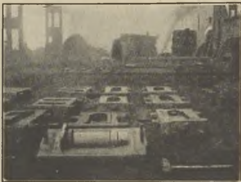
FIG. 3.—A NUMBER OF MOULDS SHOWING THE LONG PINS USED WITH COTTER HOLES.
