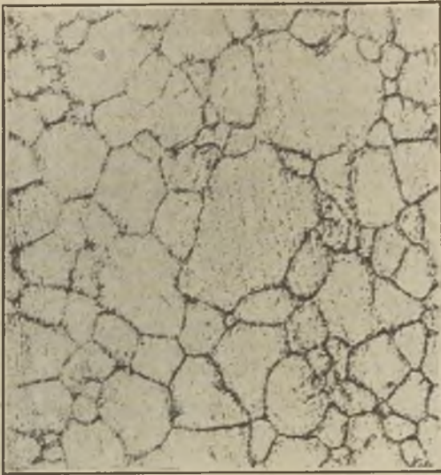
FIG. 24.—SHOWING INFLUENCE OF GASSING THE ALLOY SHOWN IN FIG. 23 (V-400-X).
