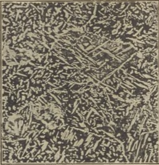
FIG. 12.—ALPHA-BETA BRASS—SPECIFICATION B (V—50—X).
