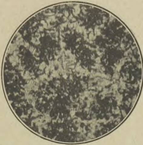
FIG. 18.—MICROSTRUCTURE OF THE INNER SECTION OF SPUN PIPE \times 100 DIAS. ETCHED 10 PER CENT. NITRIC ACID.
