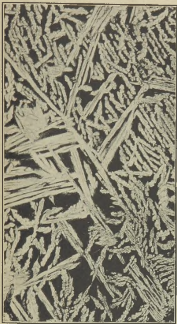
FIG. 19.—ALUMINIUM-NICKEL-BRONZE AT 50 DIAS.
