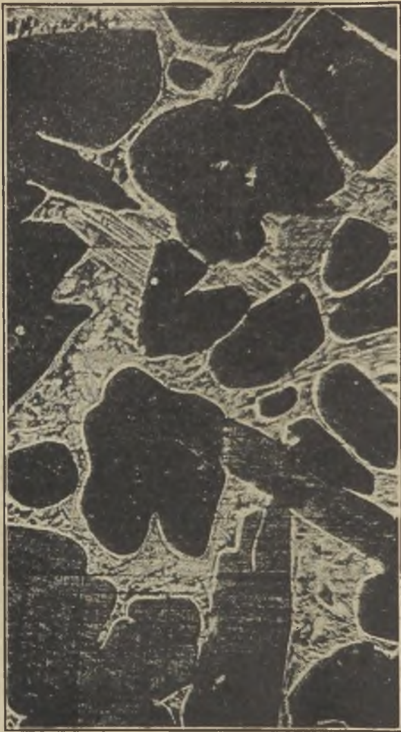
FIG. 20.—ALUMINIUM-NICKEL-BRONZE AT 200 DIAS.
