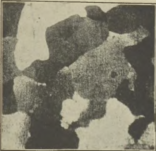
FIG. 11.—ALPHA BRASS—SPECIFICATION A (V—50—X).
