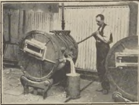
FIG. 4.—MELTING FURNACE OF THE OPEN FLAME TILTING TYPE (SELAS TURNER).
