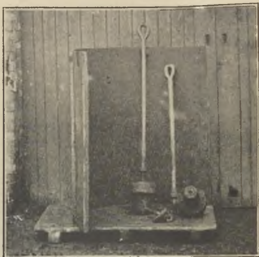
FIG. 8. C.I. CENTRING BOSS AND LONG EYE-BOLT FOR CARRYING THE CORE.
