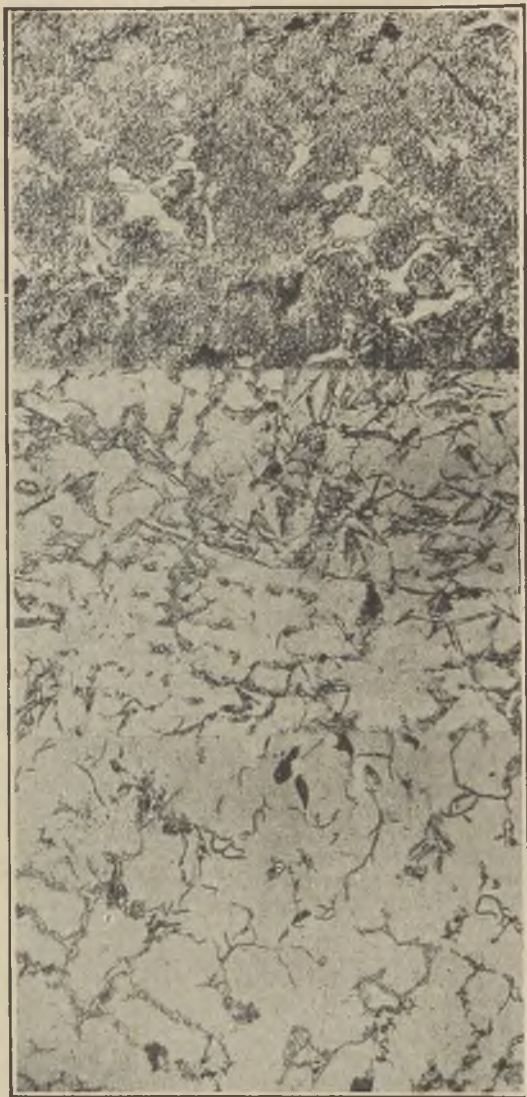
FIG. 15. SPECIMEN N3 (ANNEALED), ETCHED \times 100.
