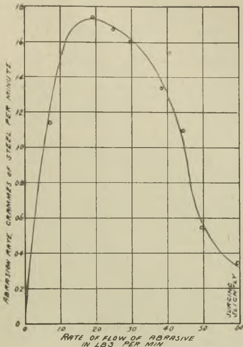
FIG. 1.—SHOWING RELATION BETWEEN FLOW RATE AND ABRASION RATE.
