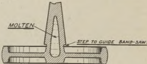
FIG. 9.—INVERTING THE RISER TO ENSURE THOROUGH FEEDING.
