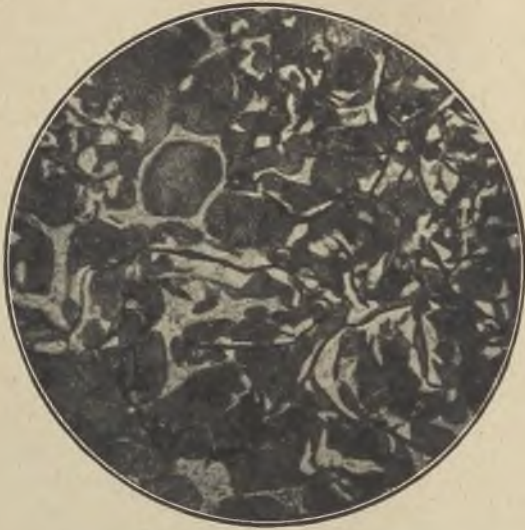
FIG. 3.—FERRITIC-PEARLITIC CAST IRON WITH THE GRAPHITE IN FINE NODULES.
