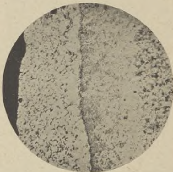
FIG. 21. \times 50 . SHOWING THE THREE ZONES IN "PEELED" MALLEABLE.
