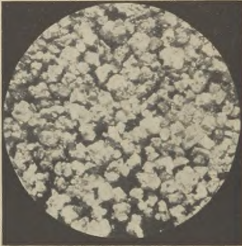
FIG. 5.— \times 25 . UNWASHED ERITH LOAM. SAND GRAINS REMAINING ON THE 120- MESH I.M.M. SIEVE=7.58 PER CENT.
