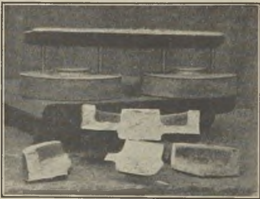
FIG. 12.—THE WHEEL BLANKS AS SEEN IN FIG. 11, SHOWING FREEDOM FROM POROSITY. NOTE THE JET RUNNERS.
