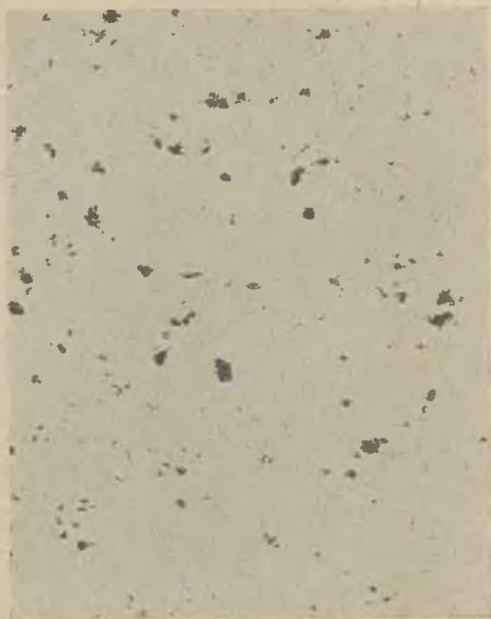
FIG. 5A.—GRAPHITE STRUCTURE FROM HEAT A VI \times 100.
