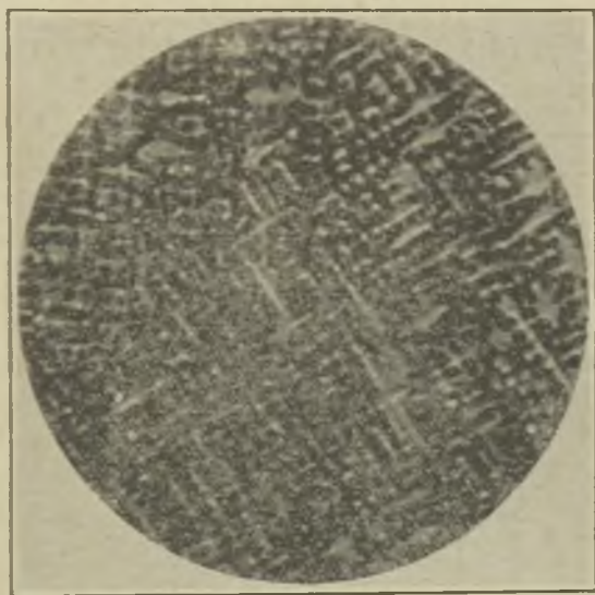
FIG. 4.—TYPICAL DENDRITIC GROWTH IN ALLOYS. COPPER-NICKEL ALLOY \times 30 .
