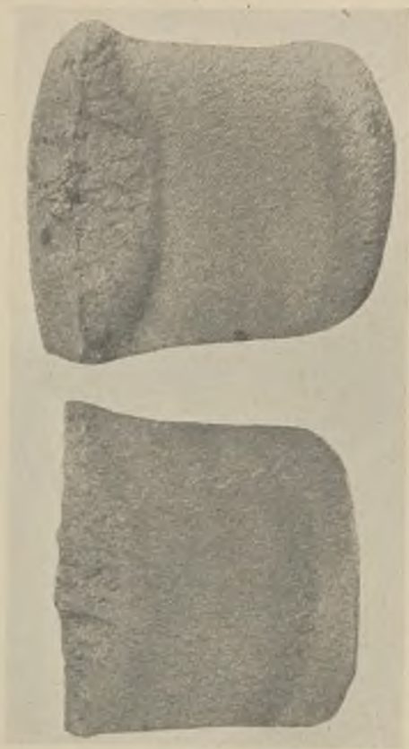
FIG. 4.—BROKEN TRANSVERSE TEST PIECES FROM HEAT BVI x 15.
