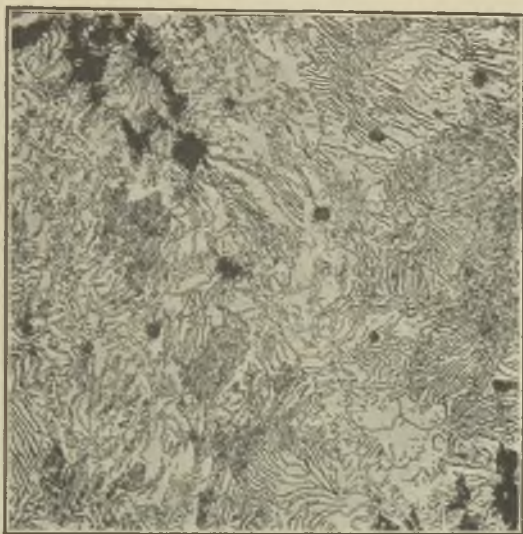
FIG. 3.—MN. 0.045 AND S. 0.014 PER CENT. ANNEALED. ETCHED WITH PICRIC ACID. × 200.
