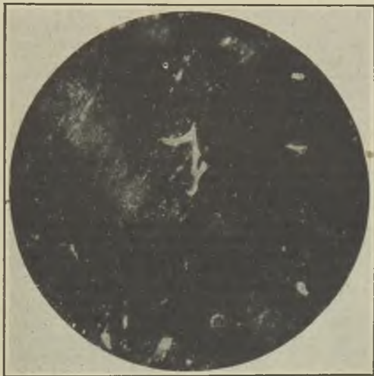
FIG. 5.—PURE 10 PER CENT. BRONZE \times 250, SHOWING COREING AND ALPHA-DELTA EUTECTOID.
