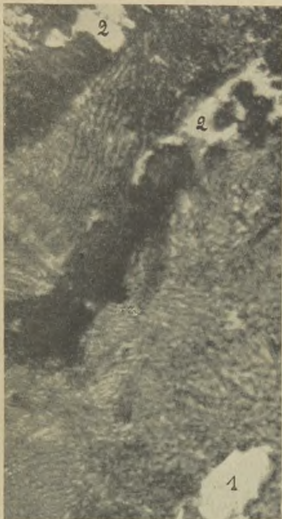
FIG. 9a.—PISTON RING IRON (1) CEMENTITE, (2) LIGHT REFLECTIONS FROM THE GRAPHITE \times 700 .
