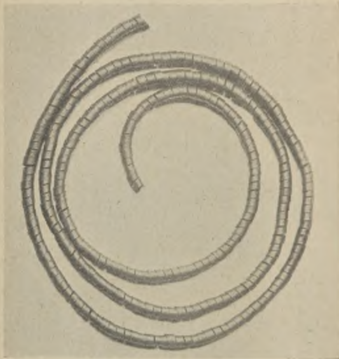
FIG. 2.—APPEARANCE OF TURNINGS SHOWING ELASTICITY—NATURAL SIZE.
