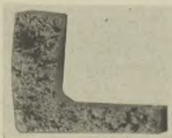
FIG. 4.—FRACTURE OF WEAK GUN-METAL. (BROKEN HOT.)
