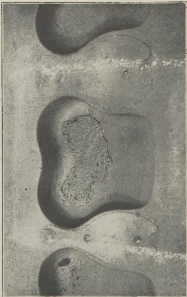
FIG. 5. SCABBED CASTINGS. CYLINDER-HEAD COMBUSTION SPACES.
