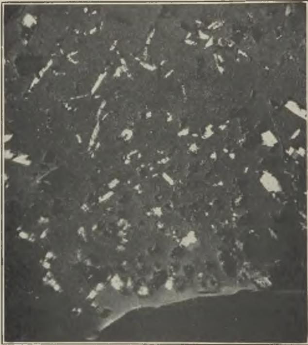
FIG. 17.—COARSE GRAPHITE SHOWN IN FIGS. 10 AND 11 VIEWED UNDER POLARISED LIGHT.
