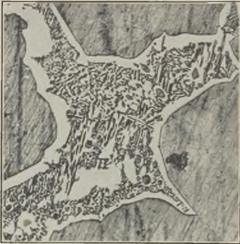
FIG. 2.—ALPHA-DELTA EUTECTOID IN CAST BRONZES.
