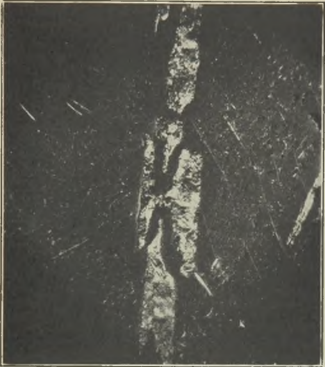
FIG. 19.—SHOWS FRACTURED GRAPHITE FLAKE VIEWED BETWEEN CROSSED NICOLS.
