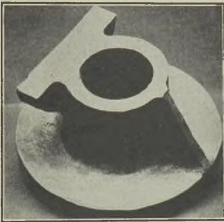
FIG. 19.—CASTING AFTER BEING BURNED-ON.
