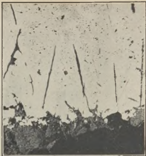
FIG. 1.—SHOWS HOW THE CRUCIBLE WALLS INFLUENCE GRAPHITE SIZE. \times 100 .
