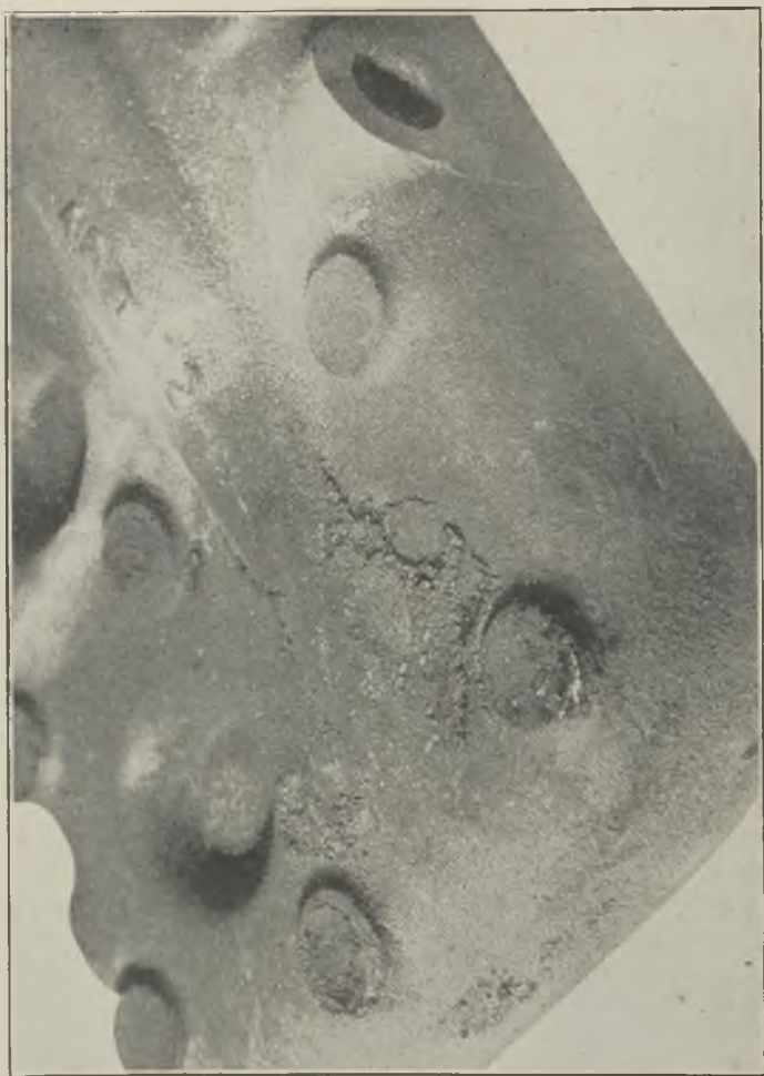
FIG. 2.—DIRTY CASTING—CYLINDER HEAD.
