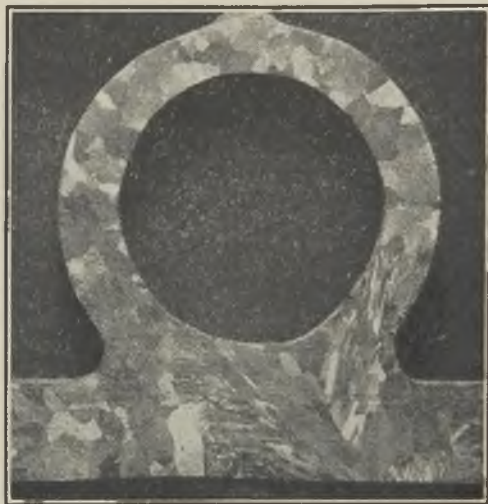
FIG. 20.—MACRO-ETCHING FROM THE REPAIRED CASTING.
