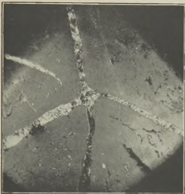
FIG. 18.—COARSE GRAPHITE FLAKES CORRESPONDING TO FIG. 7, VIEWED BETWEEN CROSSED NICOLS.
