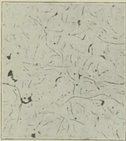
FIG. 28.—GRAPHITE STRUCTURE OF TWO CAST IRONS OF SIMILAR COMPOSITION (C 3.04, Si 2.28, AND Cu 1.92) EXAMINED BY SOHNCHEN FOR THEIR PHYSICAL PROPERTIES. (a) SAND CAST, HEAT TREATED, UNETCHED. \times 100 . (b) CHILL CAST, HEAT TREATED, UNETCHED. \times 100 .
