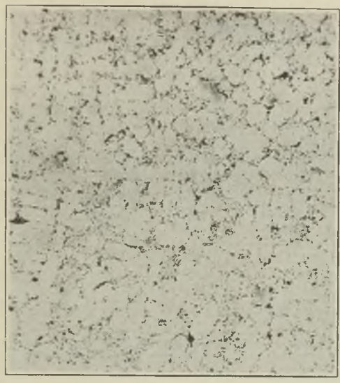
FIG. 28.—GRAPHITE STRUCTURE OF TWO CAST IRONS OF SIMILAR COMPOSITION (C 3.04, Si 2.28, AND Cu 1.92) EXAMINED BY SOHNCHEN FOR THEIR PHYSICAL PROPERTIES. (a) SAND CAST, HEAT TREATED, UNETCHED. \times 100 . (b) CHILL CAST, HEAT TREATED, UNETCHED. \times 100 .
