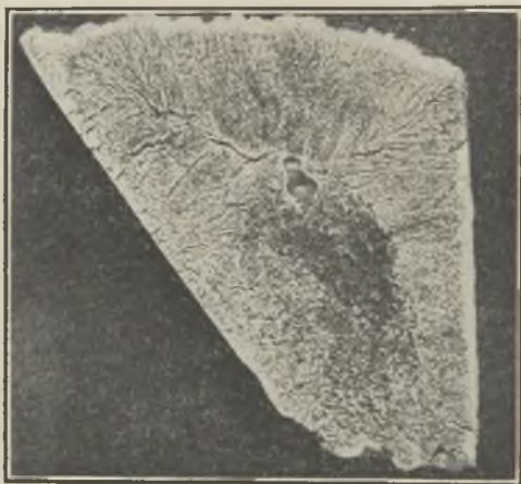
FIG. 8.—ON DEEP ETCHING THE SERIOUS CHARACTER OF THE DEFECT SHOWN IN FIG. 7 IS REVEALED.
