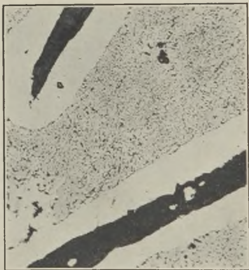
FIG. 2.—TWO GRAPHITE FLAKES (KISH) \frac{1}{8} IN. LONG, WITH FINE EUTECTIC GRAPHITE. \times 100 .
