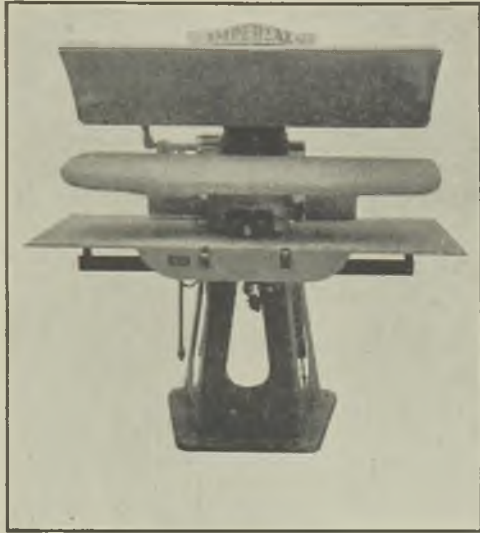
FIG. 13.—TULLIS PNEUMATIC PRESS.
