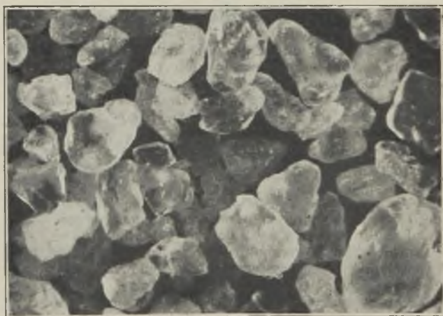
FIG. 12.—THE LARGER GRAIN SIZE OF BROMSGROVE RED SAND WASHED WITH HCL.
