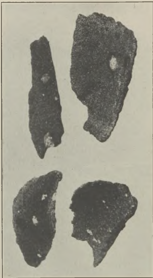
FIG. 7.—SHOWS CONDITION OF UNBROKEN CLAY PELLETS FUSED IN THE SAND MASS.
