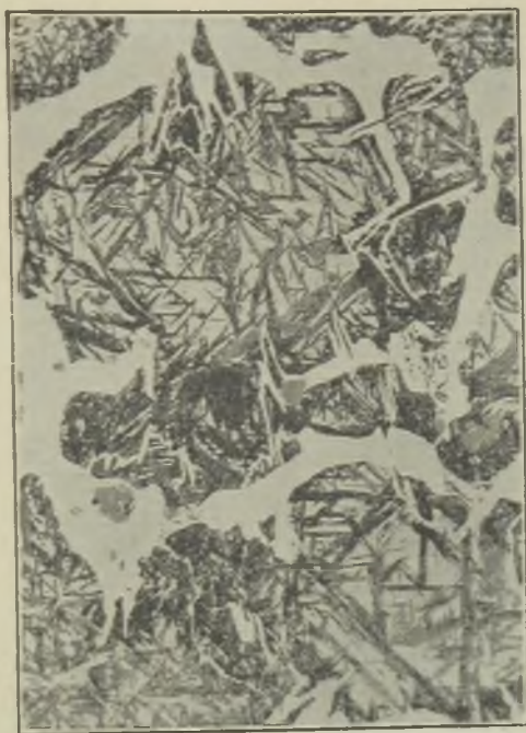
FIG. 2.—A NI-CR CHILLED CAST IRON, SHOWING MARTENSITIC MATRIX. \times 500 .
