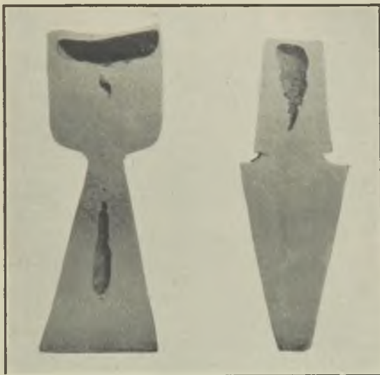
FIG. 1.—CONTRACTION AND FEEDING IN DIFFERENT TYPES OF INGOT.
