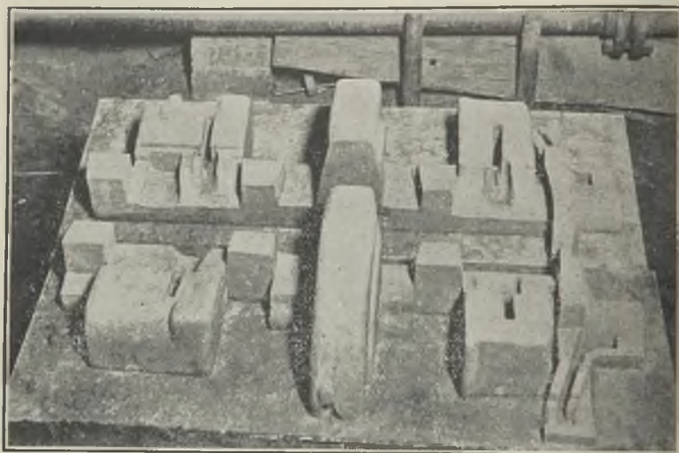
FIG. 8.—MAIN CENTRAL CORE FOR TURBINE-PUMP FRAMING.
