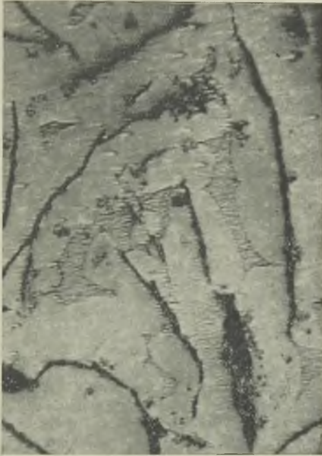
FIG. 2.—MICROGRAPH OF BADLY-WORN CYLINDER LINER. \times 110 . UNETCHED.
