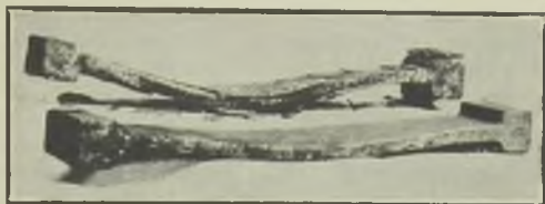
FIG. 7.—SHOWING THE SUPERIORITY OF NI-RESIST OVER SILAL FOR HIGH-TEMPERATURE KILN WORK.
