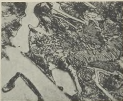
FIG. 5.—1A. AS CAST. \times 1,500 DIAS. ETCHED PICRIC ACID.
