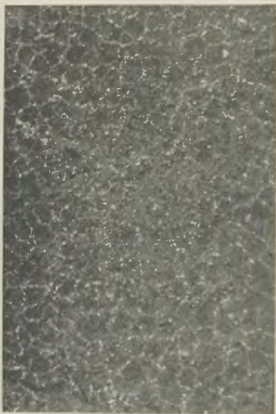
FIG. 10.—FRACTURE OF 3-IN. DIA. BAR OF IRON D (SEE TABLE II). × 1TH.
