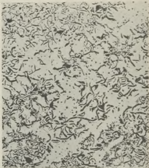
FIG. 14.—CENTRE OF CASTING. \times 50 . UNETCHED.
