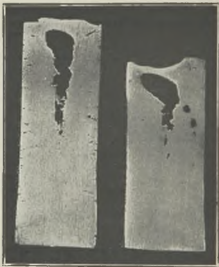
FIG. 1.—TEST INGOTS FOR ASCERTAINING SOUNDNESS.
