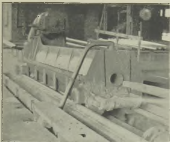
FIG. 15.—WATER-BOX CONTAINING THE MOULD.
