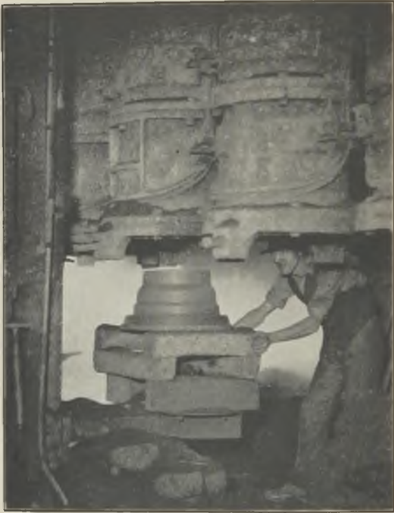
FIG. 9.—PLACING THE SOCKET PATTERN IN POSITION.
