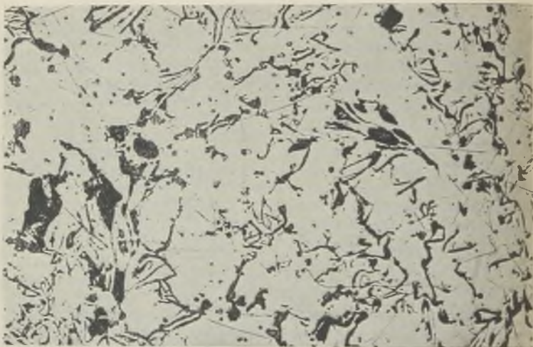
FIG. 5.—CYLINDER IRON POURED DULL. HELD IN LADLE 20 MINS. GRAPHITE AT 50 \times .
