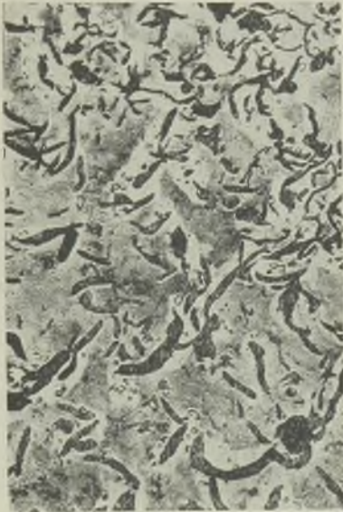
FIG. 5.—MIXED FINE AND COARSE GRAPHITE STRUCTURE OF IRON A (SEE TABLE I). \times 200 .
