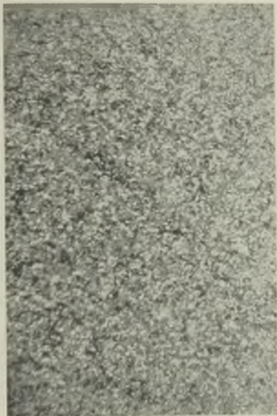
FIG. 9.—FRACTURE OF 3-IN. DIA. BAR OF IRON C (SEE TABLE II). \times 1\frac{1}{5} TH.
