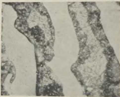
FIG. 9.—2G. AS CAST. \times 1,500 DIAS. ETCHED PICRIC ACID.
