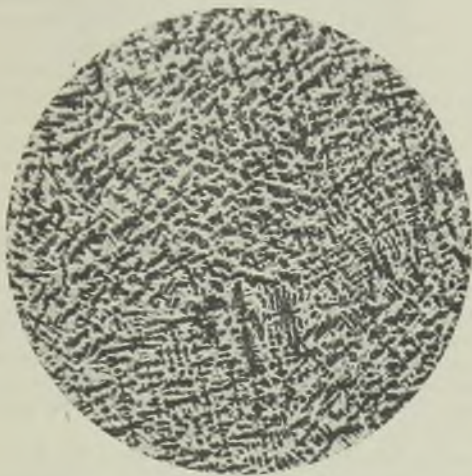
FIG. 6.—MICROSTRUCTURE OF CHILLED-STEEL ABRASIVE.
