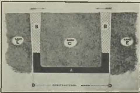
FIG. 9.—CONTRACTION ON A SIMPLE CASTING.
