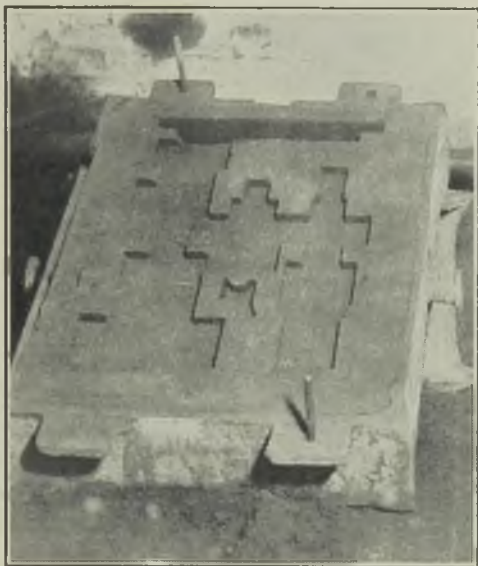
FIG. 18.—DRAG HALF OF GEAR-CASE MOULD.
