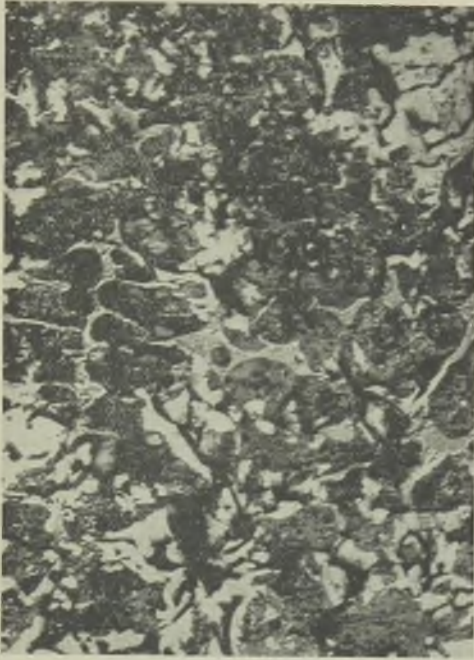
FIG. 4.—CRACKED-LINER METAL AFTER 100 HOURS' WORK. \times 110 . ETCHED.
