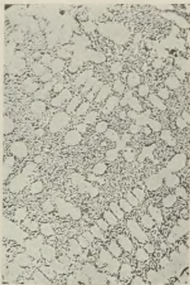
FIG. 8.—FINE GRAPHITE STRUCTURE OF IRON D (SEE TABLE II). × 50 (UNETCHED).
