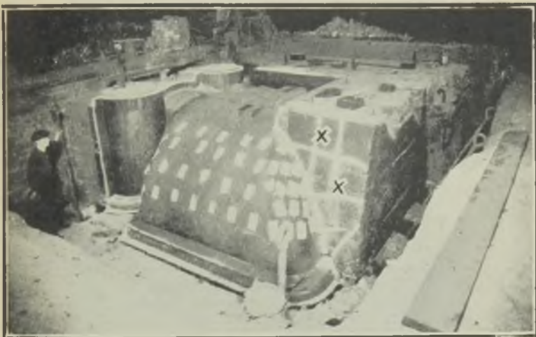
FIG. 14.—AIR CHANNELS SHOWN AT X X FOR VENTING DRAWBACKS.
