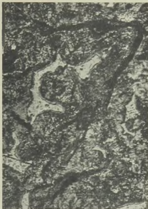
FIG. 3.—POOR-QUALITY CYLINDER LINER METAL. × 110. ETCHED.
