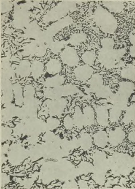
FIG. 1.—“SILAL,” SHOWING CARBON IN THE SUPERCOOLED FORM. \times 200 .
