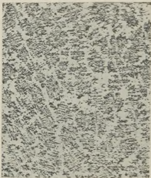
FIG. 12.—NEAR SURFACE OF CASTING. × 50. UNETCHED.
