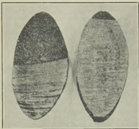
FIG. 22.—SECTIONS OF THE STRESSED AND UNSTRESSED SPOKES.
