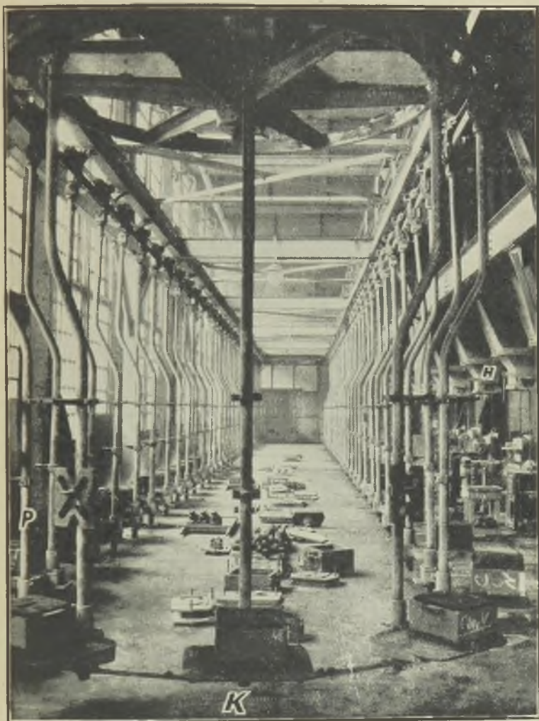
FIG. 6.—THE MOULD CONVEYOR OF THE PENDULUM TYPE.
