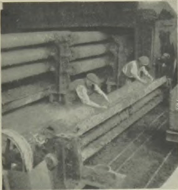
FIG. 13.--STRIKING UP THE MAIN CORE. THE FINISHED CORES AT THE REAR ARE SEEN ENTERING THE DRYING STOVES.
