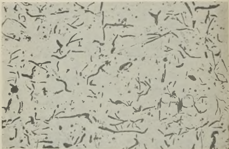
FIG. 4.—CYLINDER IRON POURED HOT. GRAPHITE AT 50 \times .
