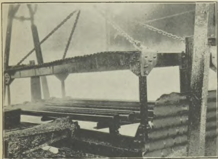
FIG. 23.—COOLING SPUN IRON PIPES.
