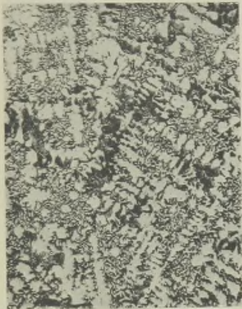
FIG. 13.—NEAR SURFACE OF CASTING. × 200. ETCHED.
