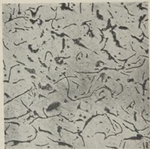
FIG. 5.—HEAT 48 AFTER SUPERHEATING. \times 100 .
