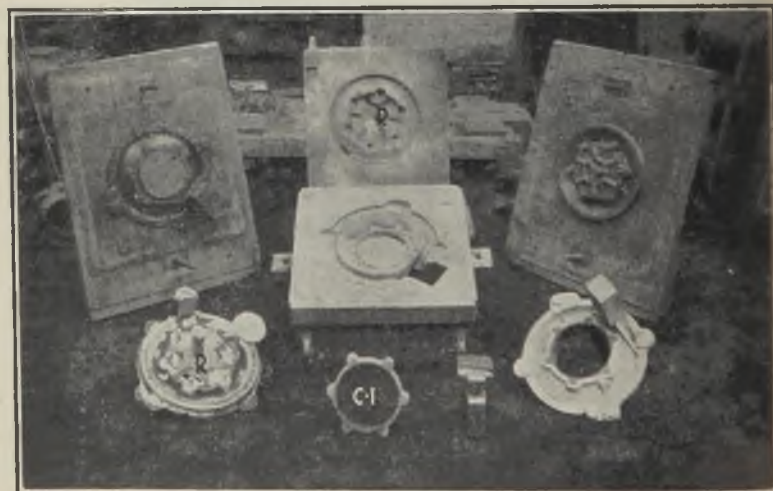
FIG. 10.—ALUMINIUM-SILICON ALLOY CASTING WITH CAST-IRON INSERT.
