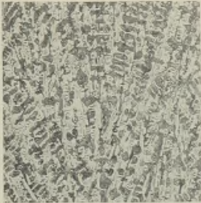
FIG. 7.—MICROSTRUCTURE OF CAM-TIP OF V-8 CAST CAMSHAFT. ETCHED 5 PER CENT. NITAL. \times 100 . (BY COURTESY OF FORD MOTOR COMPANY.)
