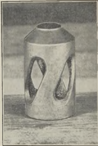
FIG. 12.—DIE-CAST VALVE PUSH-ROD, HAVING ANALYSIS: T.C, 3.65-3.90; SI, 0.30-0.65; MN, 0.15-0.50; CU, 0.75-1.0; P, 0.05 (MAX.), AND S, 0.08 (MAX.) PER CENT.
