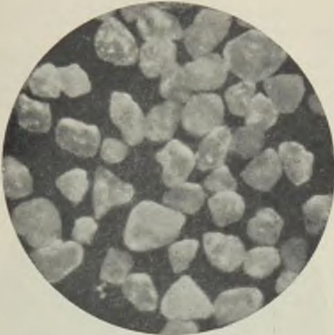
FIG. 1.—TYPICAL MICROSTRUCTURE OF BONDLESS SAND.
