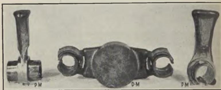
FIG. 17.—METHODS OF RUNNING PRESSURE-CAST AND PERMANENT-MOULD DIE-CASTINGS.
