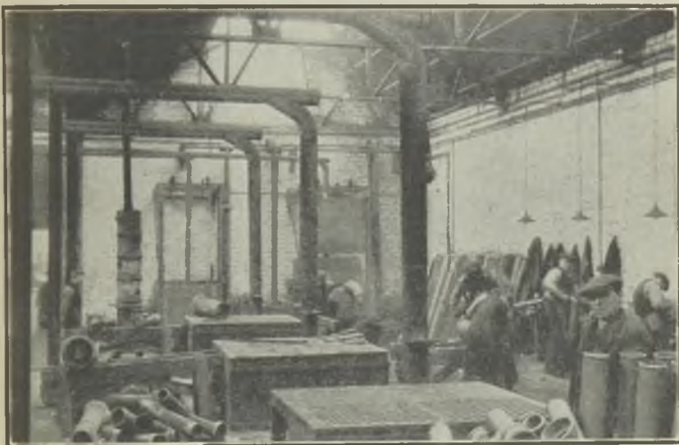
FIG. 3.—THE BRUSHING TABLES ON WHICH HEAVY AND BULKY CASTINGS ARE HAND-CLEANED.
