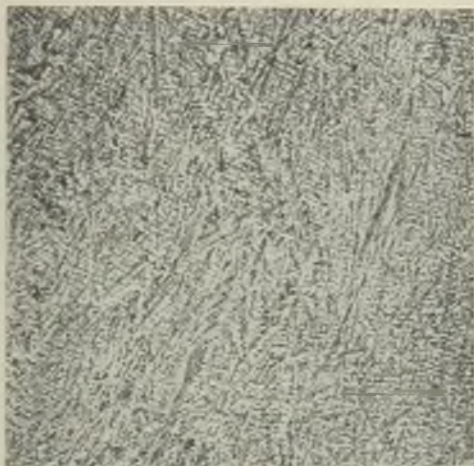
FIG. 6.—GRIT A. ETCHED IN PICRIC ACID. \times 120 .
