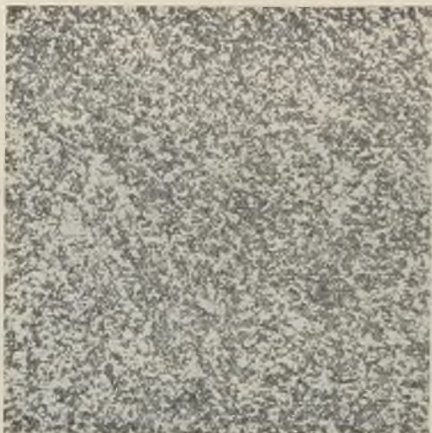
FIG. 11.—MICROSTRUCTURE OF \frac{1}{2} -IN. FORGING SHOWN IN FIG. 10. \times 120 .
