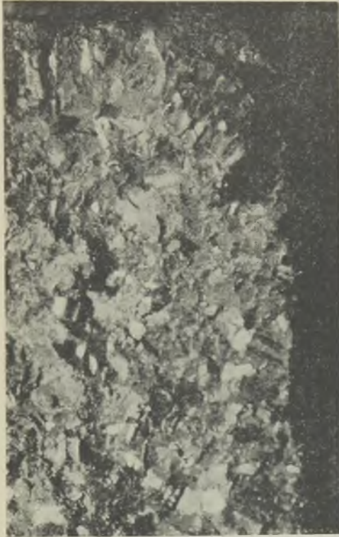
FIG. 2.—PHOTOMICROGRAPH OF SAND-CAST COPPER-CHROMIUM STEEL, SHOWING MEDIUM GRAIN. \times 5 .
