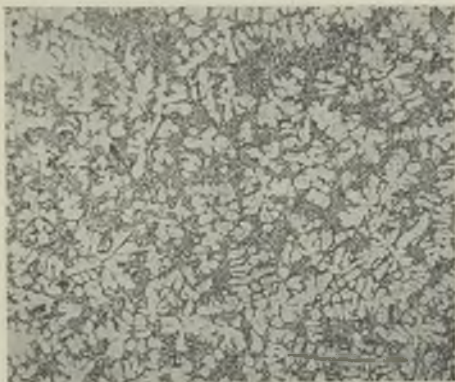
FIG. 9.—ALPAC-GAMMA WITH 10 PER CENT. SI AND 0.4 PER CENT. TI. \times 40 .
