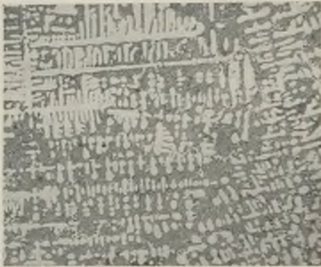
FIG. 8.—ALPAX-GAMMA WITH 10 PER CENT. SI AND 0 PER CENT. TI. \times 40 .
