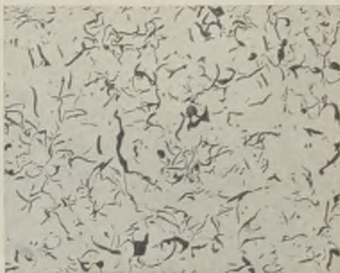
FIG. 10.—MICROSTRUCTURE OF CAST IRON SHOWING NORMAL GRAPHITE. UNETCHED. \times 50 . (B.C.I.R.A.)
