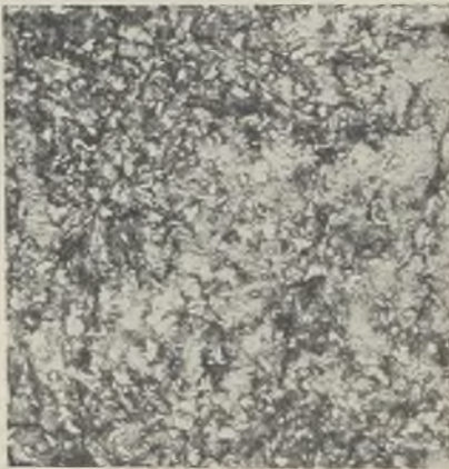
FIG. 8.—MICROSTRUCTURE OF CORE OF V-8 CAST CAMSHAFT. ETCHED 5 PER CENT. NITAL. \times 100 . (BY COURTESY OF FORD MOTOR COMPANY.)
