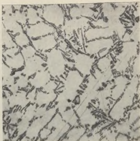
FIG. 6.—MICROSTRUCTURE OF UNMODIFIED AL-SI ALLOY. \times 100 .
