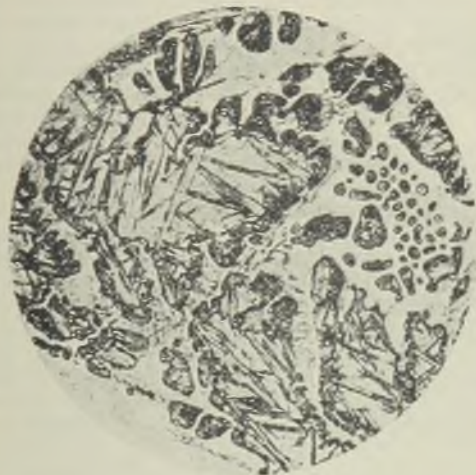
FIG. 13.—GRIT D. ETCHED IN PICRIC ACID. \times 1,200 .
