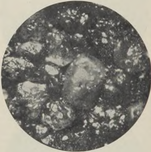
FIG. 3.—MICROSTRUCTURE OF AN IRREGULAR-GRAINED SAND.
