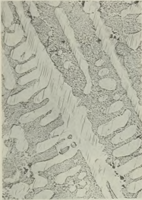
FIG. 7.—ALUMINIUM DENDRITE WITH SLIP BANDS. \times 200 .
