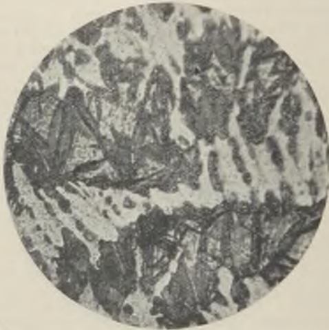
FIG. 12.—GRIT C. ETCHED IN PICRIC ACID. \times 1,200 .
