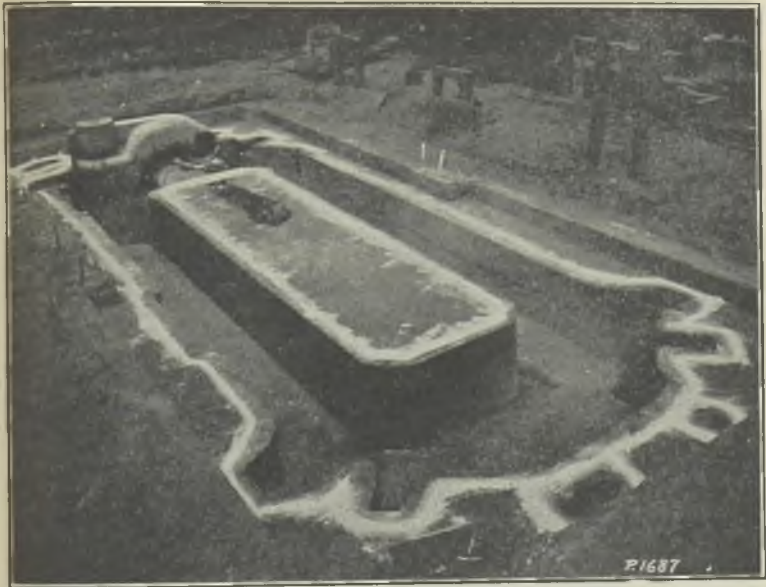
FIG. 10.—“ COMPO ” MOULD FOR MILL HOUSING.
