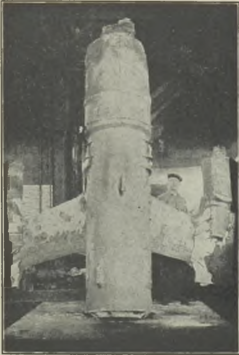
FIG. 23.—MOULD FOR LARGE STERN TUBE BRACKET IN CAST STEEL.
