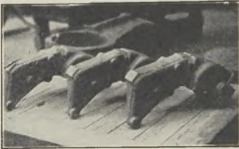
FIG. 30.—SMALL AUTOMOBILE CASTINGS MADE BY THE RANDUPSON PROCESS.
