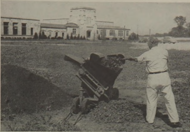
FIG. 3.—Fort Wayne, Indiana, Sewage Treatment Plant: Model "SO" Royer Sewage Sludge Disintegrator preparing sludge for use by growers, by shredding, drying, aerating and removing trash (if any, such as sticks, stones, wires, etc.) from same. This is one of 12 stationary and portable Royer models.
