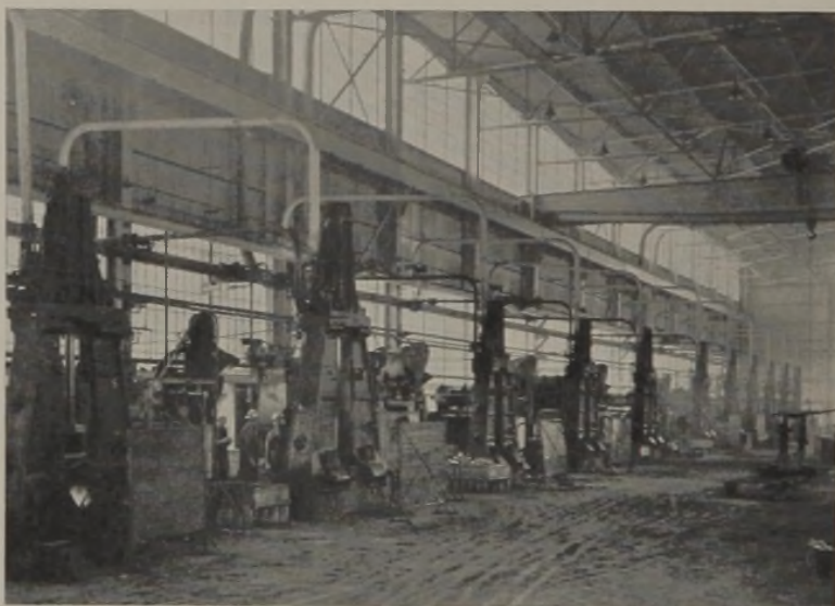
FIG. 3.—Los Angeles. Approximately 17 per cent of the aluminum going into military planes today is in the form of forgings. Aluminum Company of America has almost trebled its forging capacity at its four forging plants. At Vernon, in the midst of the airplane industry on the West Coast, there has been a 350 per cent increase in capacity. A row of 11 of the 21 hammers in that works is shown above.
