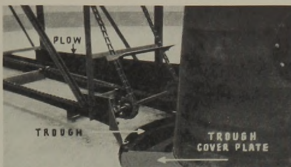
FIG. 1.—Link-Belt Circuline Collector annular covered sludge channel.
