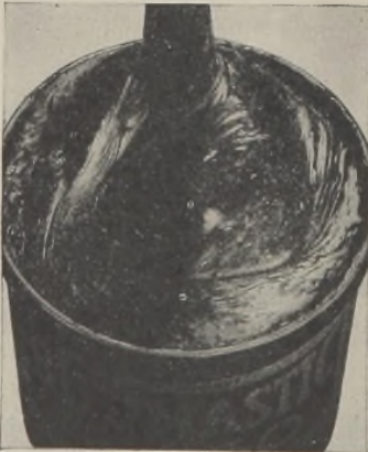
Bitumastic No. 50 thins out as it is stirred and may be applied by brush or spray.
