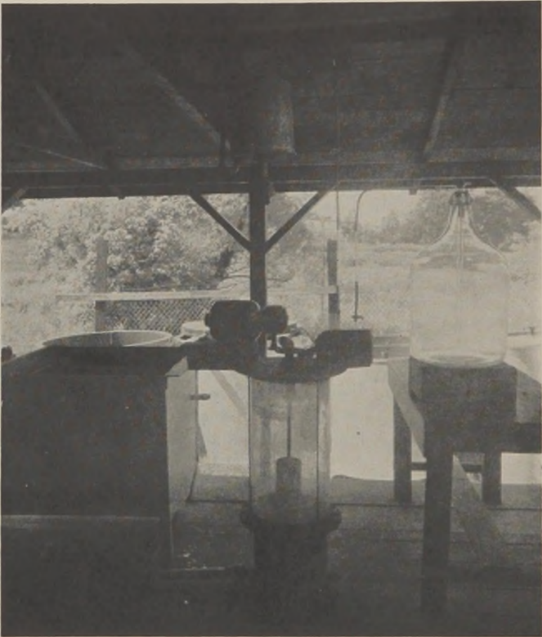
FIG. 1.—Pilot plant used for chemical precipitation of textile wastes on a continuous basis.
