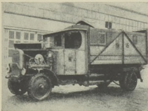
FIG. 2.—Truck equipped with sewage gas fuel cylinders.
