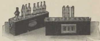
Fig. 4.—LaMotte Phosphate Comparator (Boiler Feed Water).
