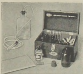
FIG. 1.—LaMotte Pomeroy Sulfide Testing Set.
