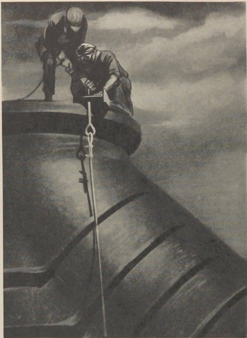
72-inch flanged Y-Branch weighing 17 tons being secured to special underslung car for rail shipment to a War Project. Drawn by Rico Lebrun for U. S. Pipe & Foundry Co.
