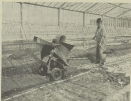
Royer Sludge Disintegrator of the type furnished the Eastern State Penitentiary of Pennsylvania—Model "NSB-2", motor driven, capacity 3 to 6 cubic yards of sludge per hour. Institutional rules prohibit showing an operating view of this Royer. One of the same model, shown below, is at work at a municipal sewage disposal plant.
