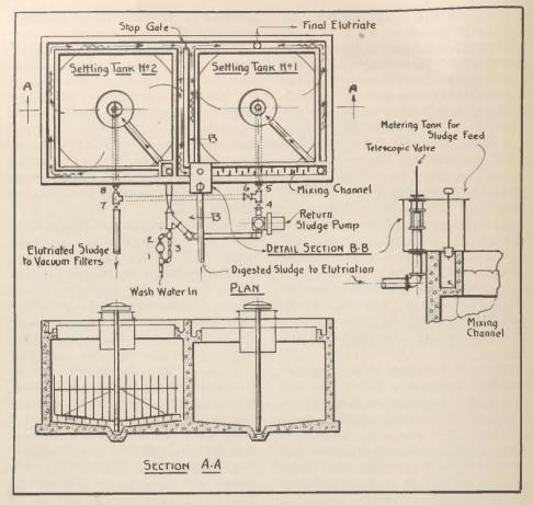
FIGURE 3.—Counter-current in companion square tanks.
