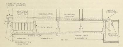
FIGURE 5 .- Cross section of grit chambers, Racine, Wis.
