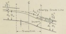
FIGURE 5.--Illustration of energy and hydraulic gradients at transition in size or grade.
