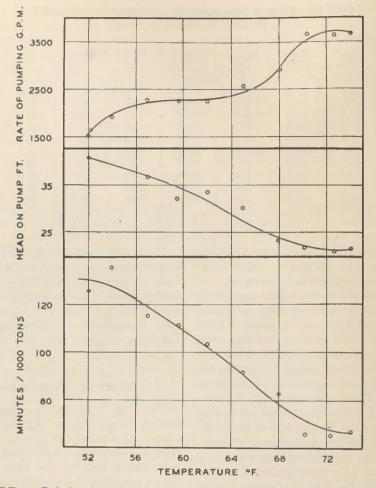
FIGURE 2.-Relation between temperature and rate and time of loading of barge.
