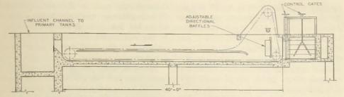
FIGURE 4.-Longitudinal section of grit chambers, Racine Wis.
