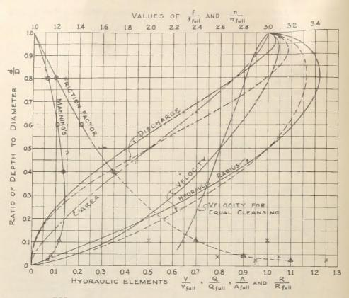
FIGURE 3.-Hydraulic elements for sewers of circular section.
