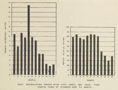
FIGURE 9.-Comparison of grit analyses made in 1939 to study effects of recirculation.
