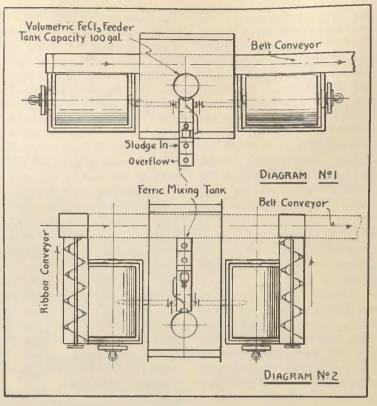
FIGURE 7 .- Feeding conditioned sludge to two filters.
