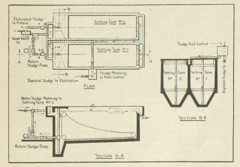
FIGURE 4.—Counter-current in companion longitudinal tanks.
