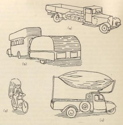
FIGURE 1.—Methods of carrying gas fuel for motor vehicles in Germany. (a) Motor truck with high pressure gas cylinders. (b) Omnibus with gas bag on roof and in supplementary car. (c) Tricycle automobile with gas bag. (d) Motor bicycle and driver with gas in knapsack.
