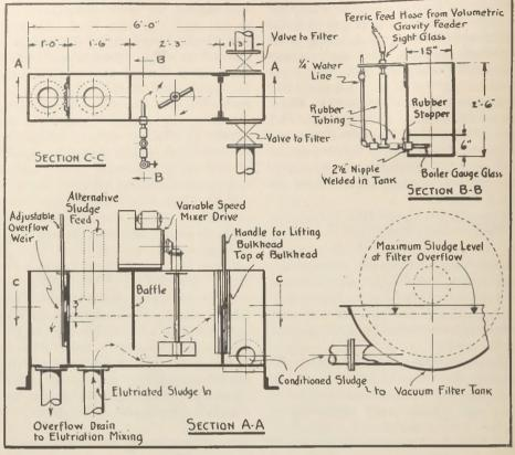
FIGURE 6.—Conditioning tank.
