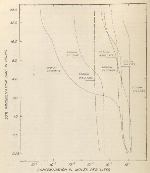
FIGURE 1.—Relation of immobilization time to concentration for Daphnia magna.
