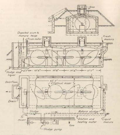
FIGURE 3 .- Digester for gasworks at farm having 50 cows.
