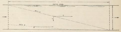
FIGURE 1.-Theoretical length of grit chamber,
