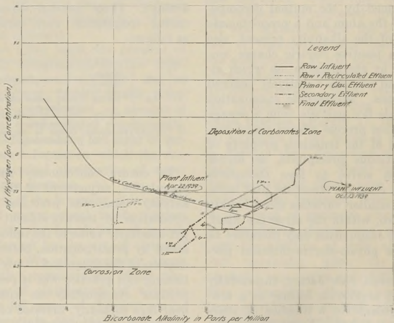
FIGURE 2.—Equilibrium curves as determined in the Ridgewood, N. J., sewage treatment plant on September 6, 1939.
