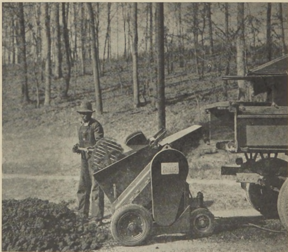
FIGURE 2.—Royer Sludge Disintegrator converting sludge into fertilizer at Charlotte, N. C.
