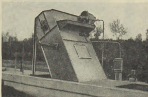
Tritor Screen. A combination screen and grit chamber for medium and small size plants. Folder 1587.
