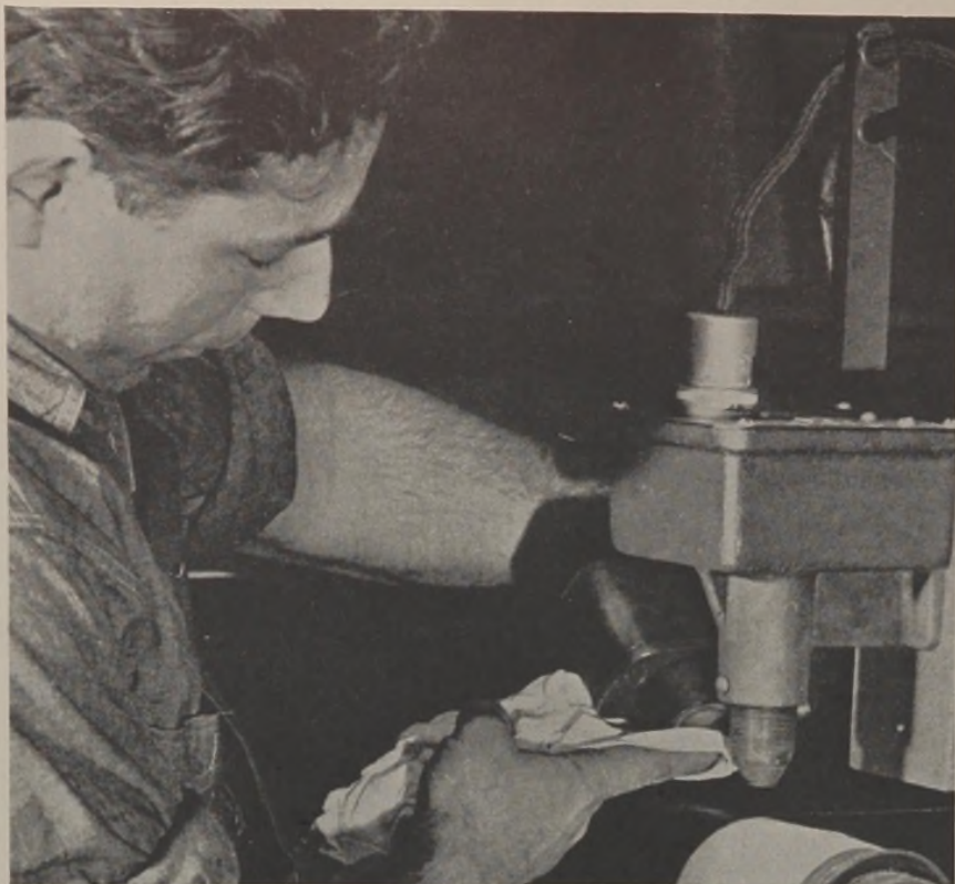
Above. Lenses and other parts of photoelectric optical systems should be cleaned regularly with soft cloth.
