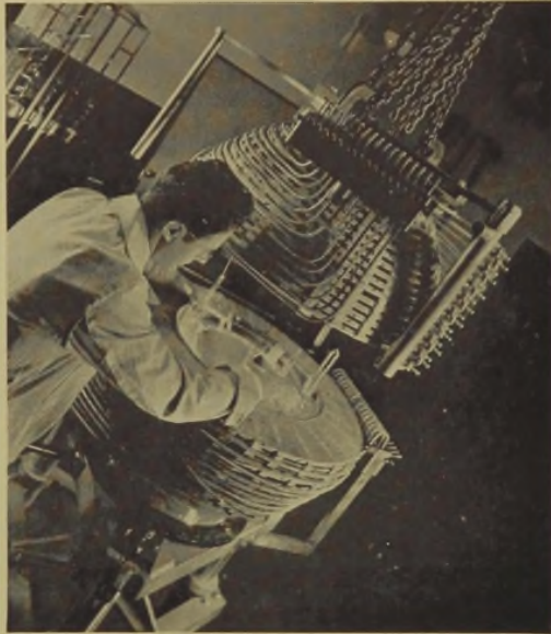
Mass spectrograph segregates gas molecules and their constituent atoms according to their masses.
