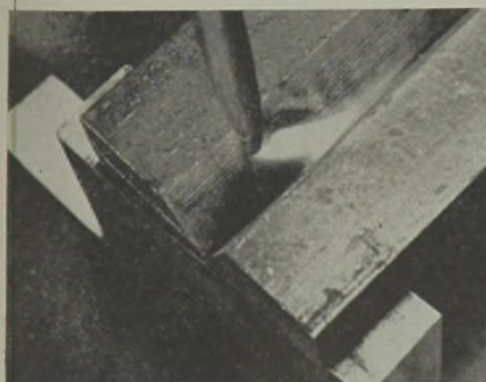
Figure 14—Arc blow at end of joint.
