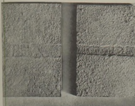
Figure 12—(left) Corrosion of welded joint ( \text{HNO}_3 ). Note weld is almost comparable to parent metal. (right) Improper electrode causes poor corrosion resistance of weld ( \text{HNO}_3 ).
