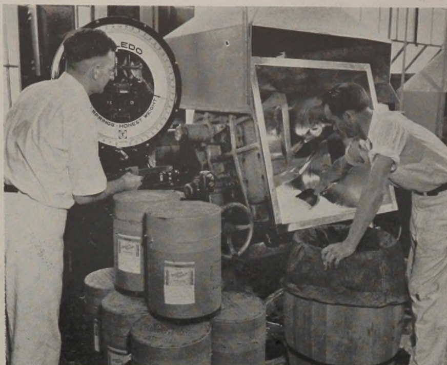
A qualified compounder makes a final check on all ingredients for a batch.
