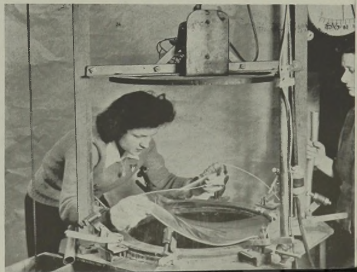
After cooling, the finished astradome is removed from the vacuum pot. It is then carefully inspected for optical and other properties before it is packed and shipped.
