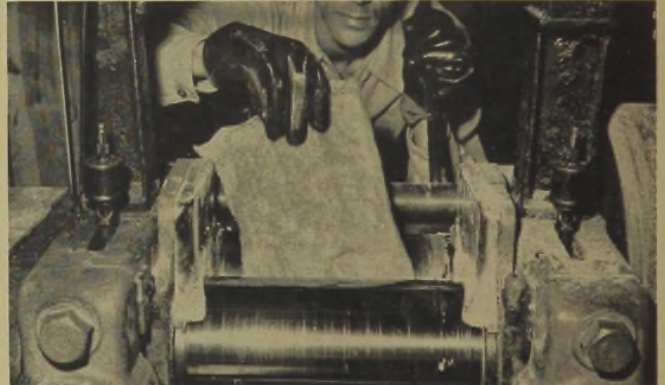
This mixing mill, a smaller twin brother of the blenders of industry, mauls between its rolls a sheet of Cerex.
