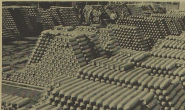
OXYGEN FOR AIRMEN: High altitude flying has tremendously stepped up need for oxygen, and mass production of cylinders is big business. Acres of them are stacked at plant of Walter Kidde & Company in New Jersey.
