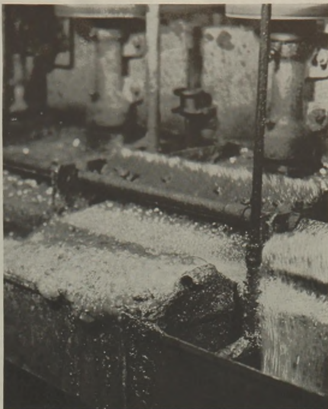
The finely divided resin-rubber agglomerate is separated from the mill slurry by flotation.
