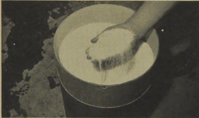
The feel and texture of Cerex is like powdered soap. This material will next go to mixing mills and then flakers.
