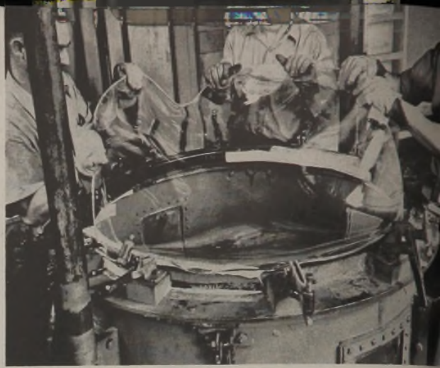
Sheets are taken from oven after heating. Thoroughly limp and flexible, they are clamped between a Masonite die-stock ring and the top flange of the vacuum pot.
