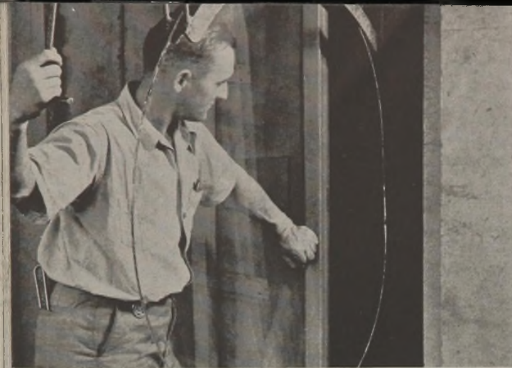
First step in "snap-back" forming of a bomber turret: flat sheet of Plexiglas, hung by spring clips, being rolled into hot-air oven at temperature of 220-300° F.
