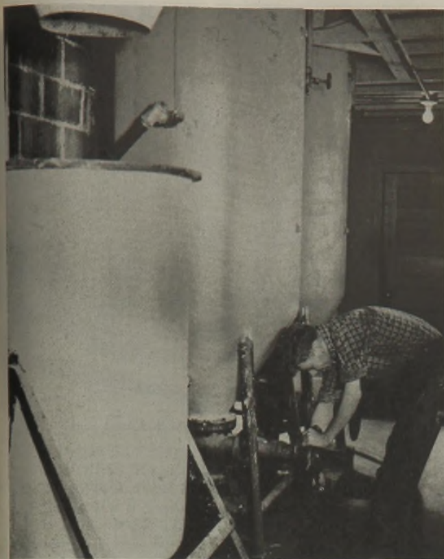
Open cooker and two pressure cookers. First step is to charge these with dried milkweed leaves and water.
