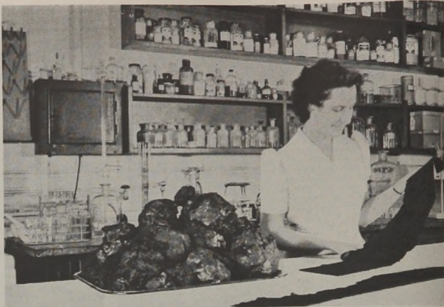
Crude lump resin-rubber gum out of the ball mill and sheeted dried gum.
