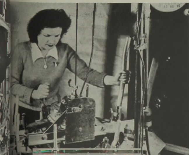
After heated sheet is clamped across pot, the valve is opened and the sheet drawn to the proper depth. A fan in the hold-down ring speeds cooling.
