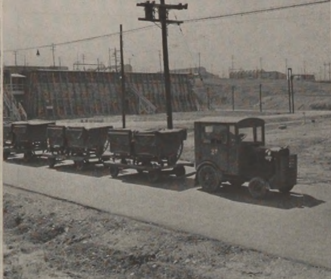
Fig. 1—Trucks are used to move bulk material between operations at a smokeless powder plant. Continuous conveyor would permit propagation of explosion or fire from one building to another.
