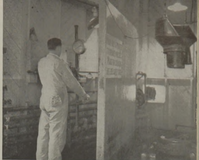
Fig. 5—Operation by remote control is one of the best safety precautions. Here an operator is protected by a steel shield while he applies pressure to a powder press.
