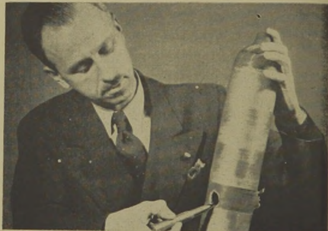
A NEW METHOD of preventing "shrapnelling" of oxygen and carbon dioxide cylinders has been developed by Walter Kidde & Co. Untreated cylinders can explode into pieces when hit by flak or bullets but wrapped with wire the cylinder is cleanly pierced.
