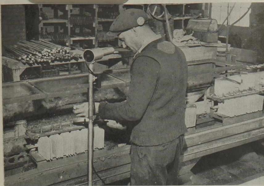
Sampling air for lead fume content with an electrostatic precipitator.
