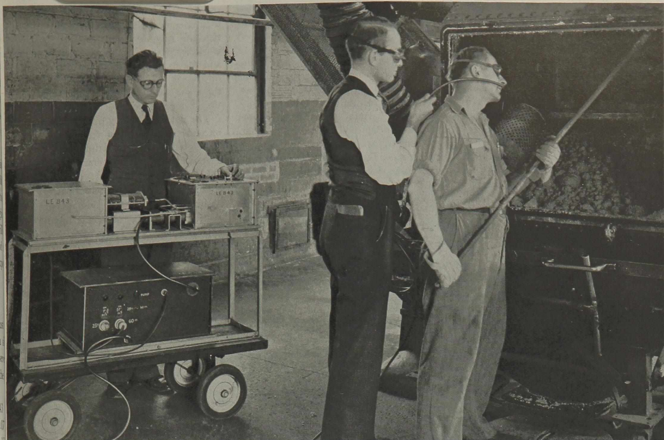
Carbon bisulfide vapor concentration is being measured by an ultraviolet photometer.
