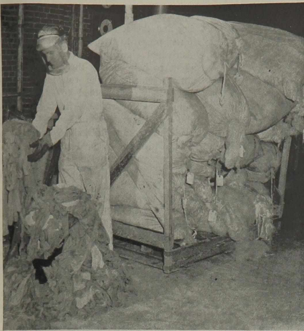
the hopper of the new nylon reclamation unit constructed at the Du Pont nylon plant at Seaford, Del.
