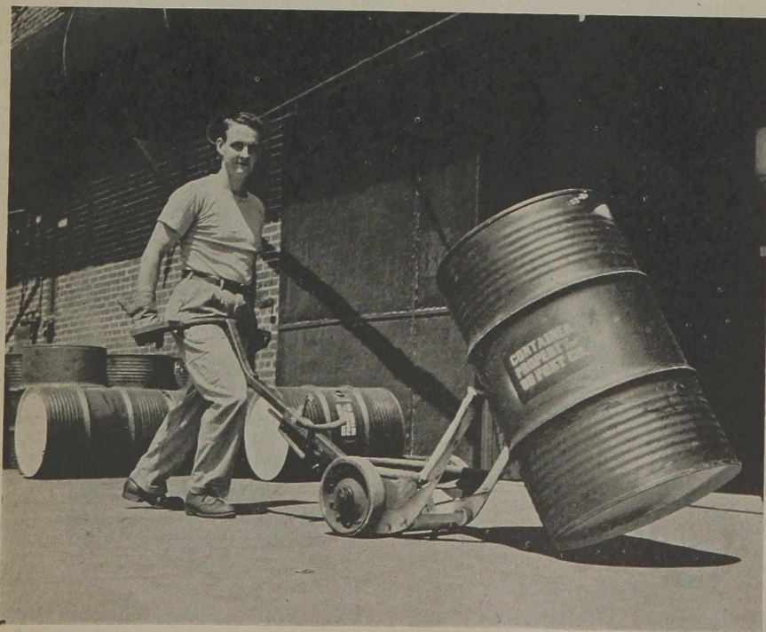
Alvin H. Potter, who devised the drum up-ender shown here, demonstrates the labor-saving device at the du Pont Toledo Finishes Plant.
