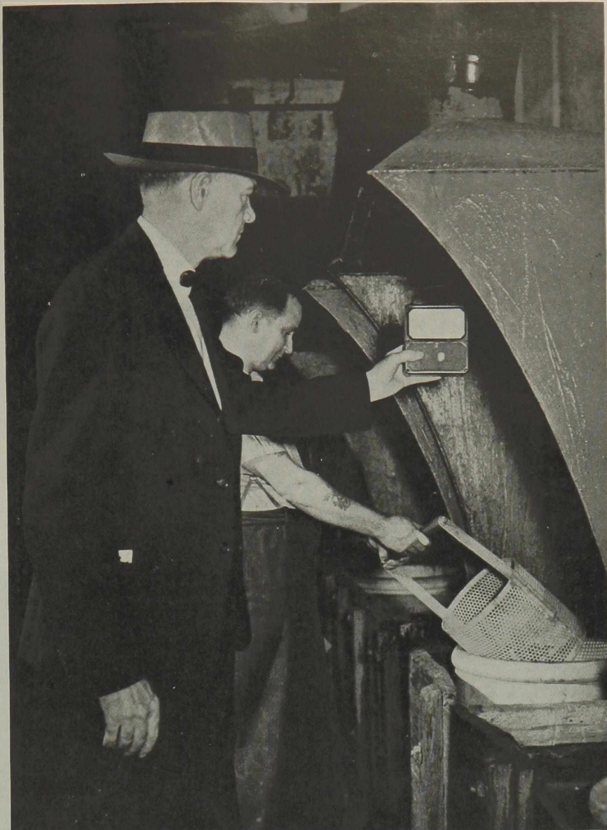
Measuring air velocity at the face of an exhausted hood. Hoods should be checked often for leaks or other faults.
