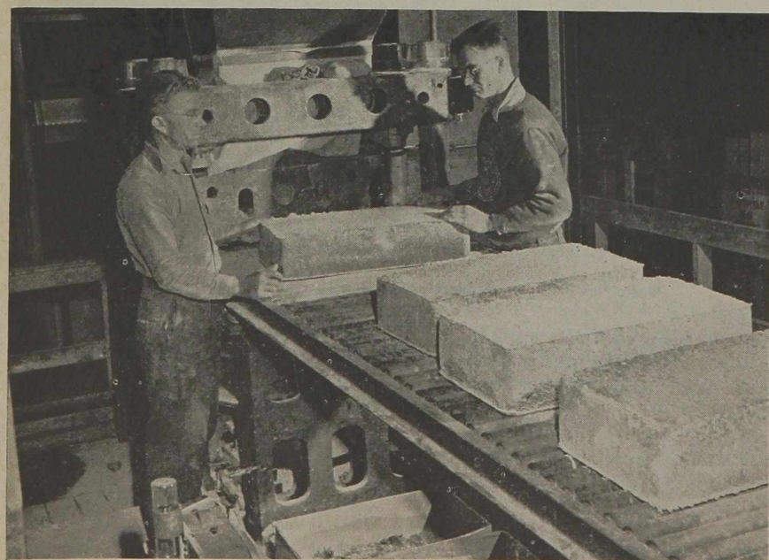
Each of these 75-lb. bales of crude Buna-S represents about 19 lbs. of styrene and 56 lbs. of butadiene.
