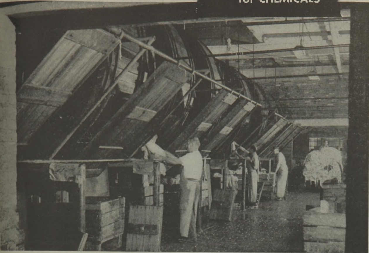
Removing sheepskins from tanning drums
