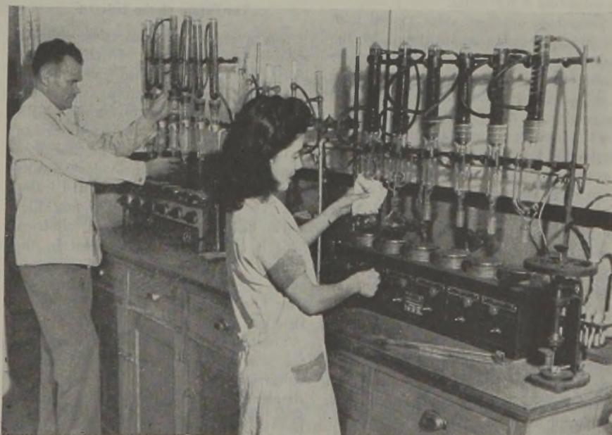
Determination of grease content of leather by Soxhlet extraction. A. C. Lawrence Leather Co.
