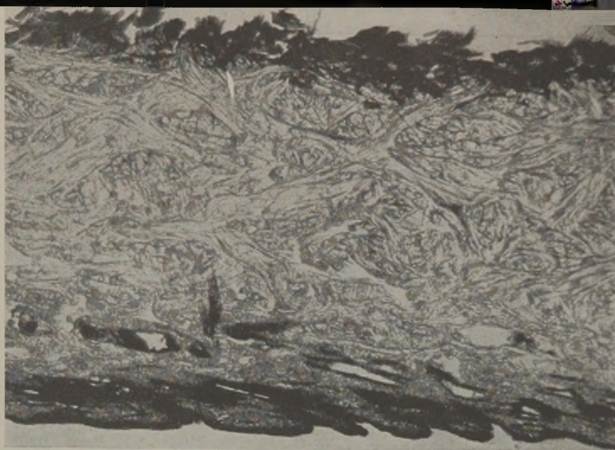
Cross section through calfskin, by M. C. McDonald, A. C. Lawrence Leather Co. Mag. about 85 X.
