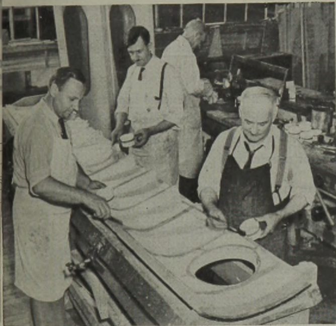
(Above) WOODEN SUB-ASSEMBLIES for the Mosquito bomber are formed into wings and fuselage, spars fastened to ribs and ribs to skin, with a bond of cold-setting BETLE Cement.
