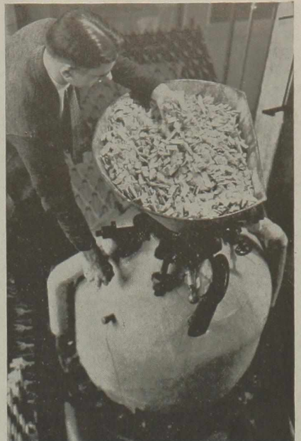
Illustration courtesy Forest Products Laboratory An experimental digester of chips for the production of lignin plastics.
