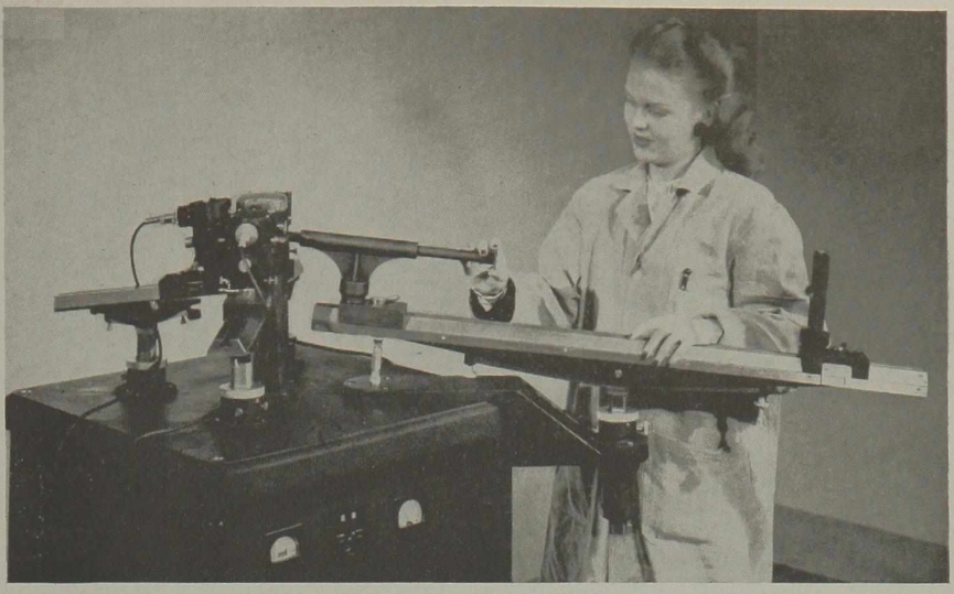
Illustration courtesy North American Philips Co. Instrument designed to measure low-angle X-ray diffraction.
