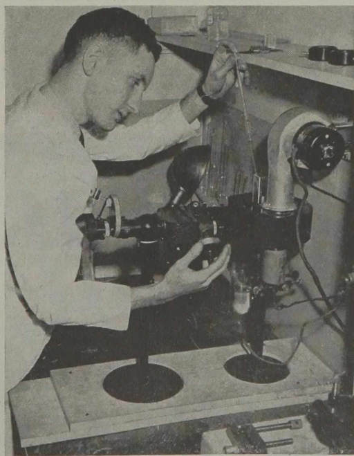
Richard Stein, Polytechnic Institute student, determines molecular weight with the Turbidimeter.
