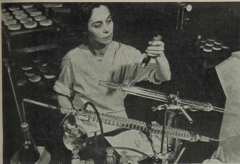
The phosphorescent character of cathode ray tubes is so sensitive to impurities that every precaution must be taken to ensure absolute cleanliness. Here the oil from the oil diffusion pump used to produce the high vacuum is distilled to remove foreign material.
