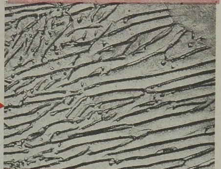
Lamellar Precipitation in a Magnesium Aluminum Alloy. X4,750
