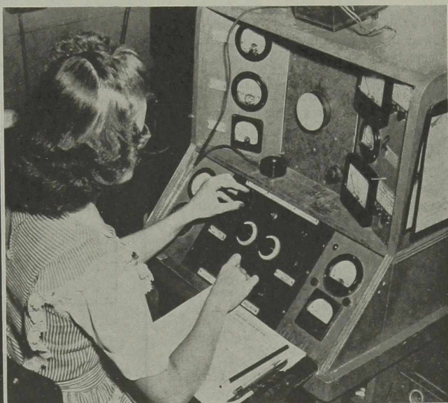
Electrical characteristics and light output of a complete 3" tube are being tested. Alignment, uniformity of cathode surface, and screen condition are a few of the items checked.
