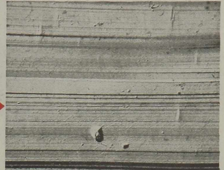
Natural Surface of a Magnesium Single Crystal grown from the Vapor Phase. X4,750
