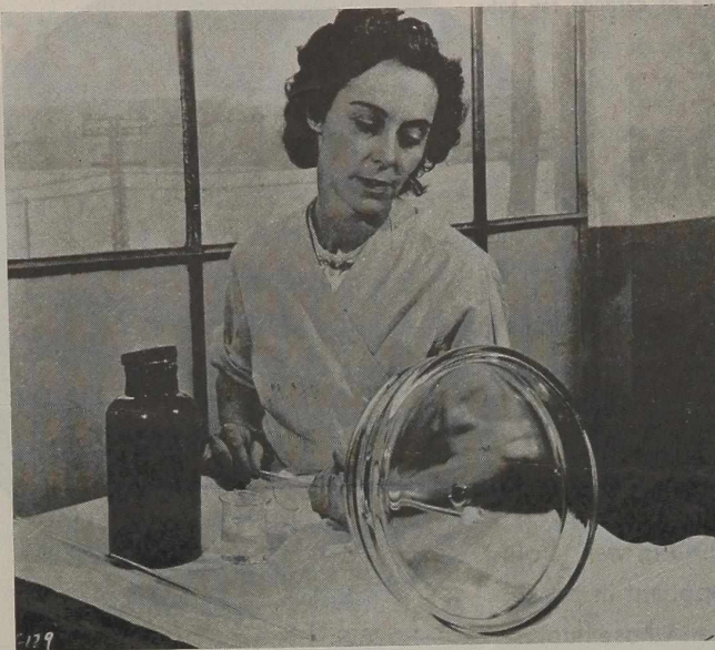
A phosphor is being applied to a 10" cathode ray tube. The glass shell has been washed, dried, and moistened with a binder. After the phosphor is dumped, the tube will be shaken to distribute the powdered material uniformly over the surface of the glass.
