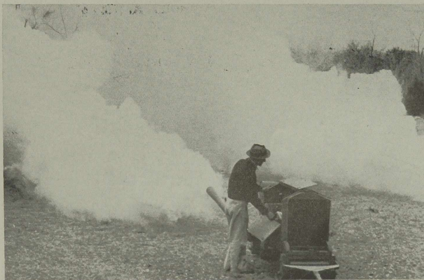
Petroleum-smoke generator being used to protect sugar-cane from frost damage.
