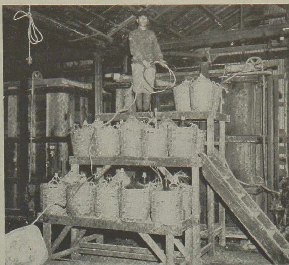
Fig. 7. Crude Japanese mixing tank for sulfuric acid and ammonia. The ammonia cylinder is shown at the lower left hand corner with a flexible tube leading to the worker's hands. Note the corrugated metal construction.
