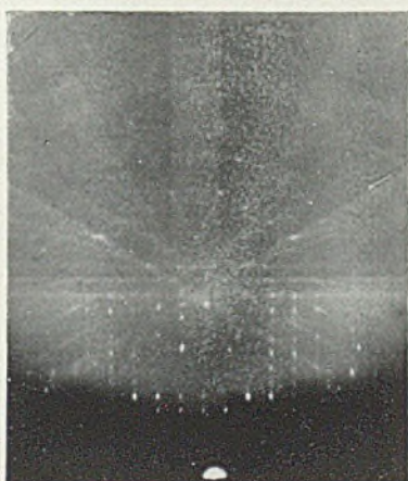
FIG. 19.—Pattern from specimen of Fig. 18 with a thin film of nickel aluminate on the surface.
