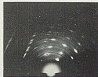
FIG. 12.—Nickel oxide on a plane of corundum inclined by 30^\circ to the basal plane. [100] azimuth of corundum, [11 \bar{2} ] of nickel oxide. Cf. Fig. 7.
