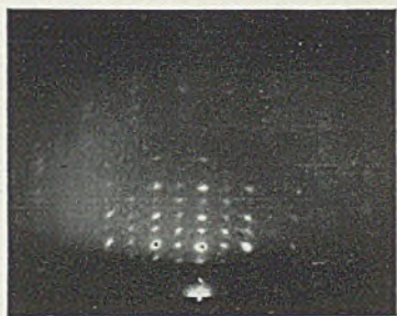
FIG. 16.—Pattern from specimen of Figs. 7 and 8 after heating, \langle 11\bar{2} \rangle azimuths of nickel oxide and aluminate.
