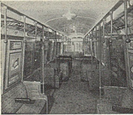
One of the experimental fluorescent lighting installations in a Metropolitan Line coach. The centre lamps are for emergency purposes
