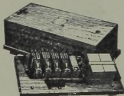
A.T.M. Auto Repeater (with cover removed)
