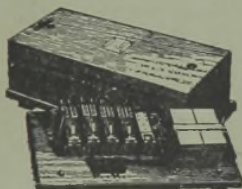
A.T.M. Auto Repeater (with cover removed)
