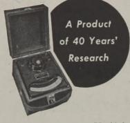
Built with the ENGELHARD frictionless galvanometer, eliminating bearings and pivots.
