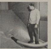
Commonly used for unloading fine, crushed and granular materials from cars and ships; reclaiming from bulk storage. Saves difference in cost between bag and bulk shipments, handling and storage. One man can operate the system.
