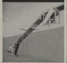
Reversible—this "Streamliner" Belt Conveyor operates either up or down at constant speed of 45 feet per minute. Its rollers can be "SET HIGH," for oversize packages, or "SET LOW" to provide a protective guard rail on both sides of the durable rough top rubber belt. Unit is available in standard sizes up to 30" wide . . . has manual take-up for belt slack . . . may be equipped with casters for portability . . . or can be supported from one floor. Write for full information.
