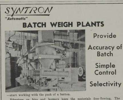
Vibrators on bins and hoppers keep the materials free-flowing, The vibratory feeders automatically filling scale hoppers to exact weight, and discharging onto secondary vibratory feeders, smoothly emptying each accurately weighed batch into mixers, blenders, belt conveyors, etc.
