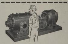
**ROTARY COMPRESSORS**, sliding vane type. Air is compressed in cells formed by blades moving freely in and out of longitudinal slots in rotor eccentric to its casing. Quiet, smooth operation. Units start unloaded. Capacities for 5 to 35 psi-g.
