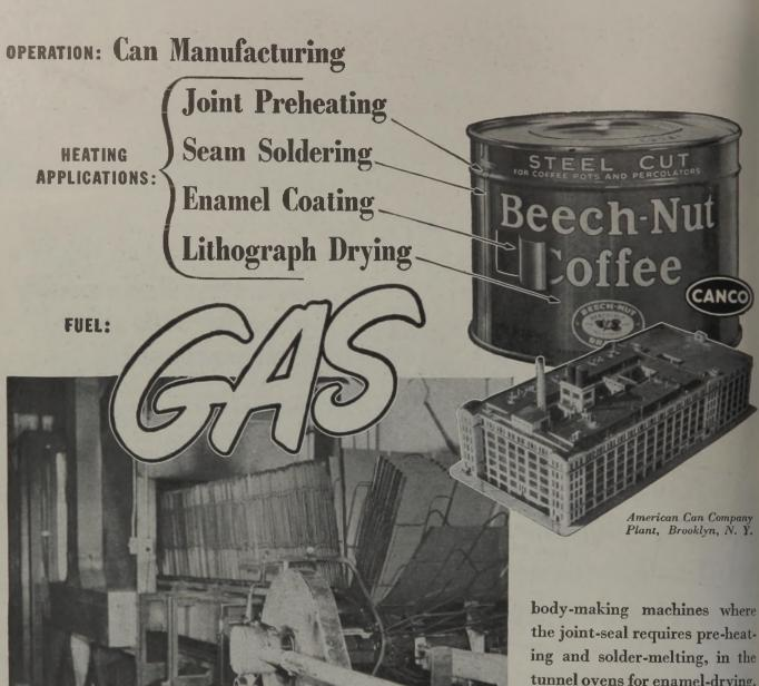
Enamel-coated tinplate emerging from drying oven
