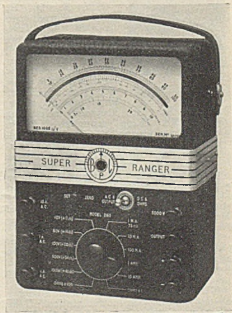
A new a.c.-d.c. multi-range tester, made by British Physical Laboratories
