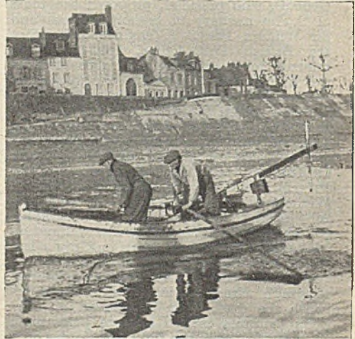
A magnetic locator being used to search for sunken buoys and shipping in the River Seine
