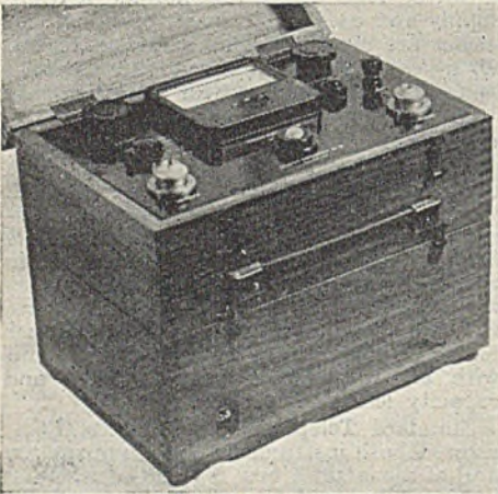
The Baldwin-Farmer electrometer, designed for radiological work
