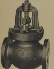
Large Iron Body Bronze Mounted Globe Valve for 125 pounds W.S.P. Made in sizes 2" to 16", inclusive. Has outside screw rising stem, bolted flanged yoke and regrindable, renewable bronze seat and disc. Also available in All Iron.
