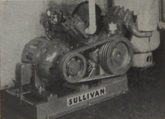
A compressor for every standard electric motor rating. More air per motor horsepower because each compressor is matched with a standard motor rating from 15 to 100 H. P. Built-in oil cooler for greater economy. Directconcentric valves for highest efficiency.
