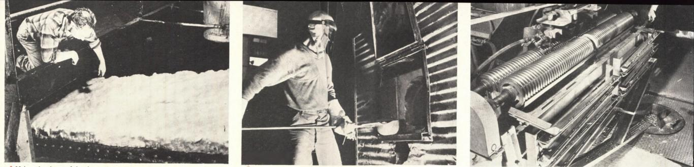
4 Molten glass is extruded and steam jets stretch the filaments while in the forming chamber. Here they are shown emerging from the chamber on a conveyor
