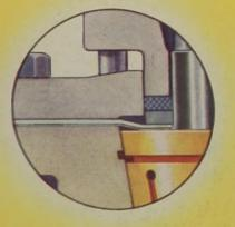
DIAPHRAGM SHOULDER SEAL This proved design provides against shank leakage with minimum friction. The ground surface at the top of the plug slides freely against a metal diaphragm.
