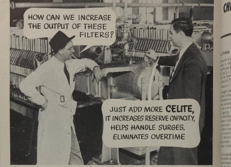
U<sup>SERS</sup> FIND that Celite\* often saves the cost of additional filters. To increase filtering capacity for peak requirements, they merely increase the proportion of Celite to the fluid until the emergency has passed.
