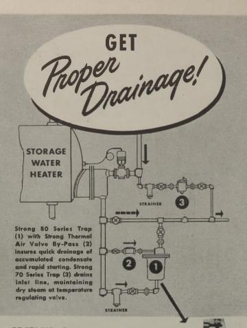
**PROBLEM:** Condensate accumulates in coils due to lack of pressure when thermostatic regulating valve is throttling or closed. *Improper drainage and water hammer result when thermostatic valve opens.*
