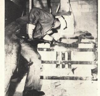
3 In this furnace the hatch-sand, limestone, and mineral oxides-is melted and refined
