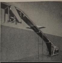
THIS STREAMLINER 30° INCLINED BELT CONVEYOR SPEEDS FLOOD TO FLOOD
